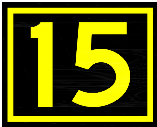
(b) Runway Location Sign
