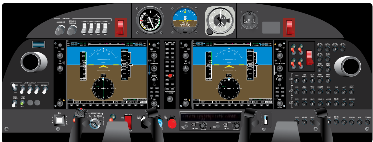
Figure 11-70. A modern glass flight deck on a general aviation aircraft. Digital data displays replace many older instruments and indicators of the past.
