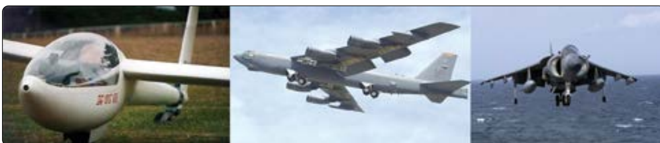
Figure 13-5. Tandem landing gear along the longitudinal axis of the aircraft permits the use of flexible wings on sailplanes (left) and select military aircraft like the B-52 (center). The VTOL Harrier (right) has tandem gear with outrigger-type gear.
