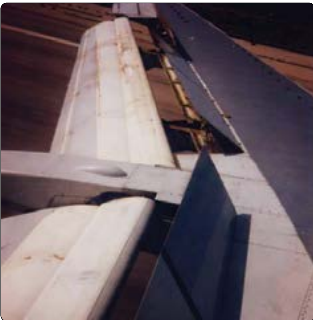
Figure 1-68. Spoilers deployed upon landing on a transport category aircraft.
