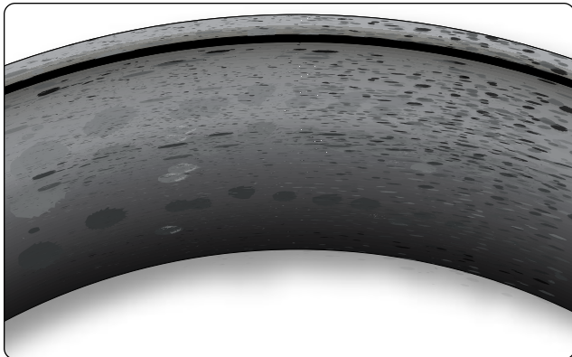
Figure 13-72. Bruising is caused by fine particle contamination possibly from a bad seal or improper maintenance of bearing cleanliness. It leaves a less than smooth surface on the bearing cup.
