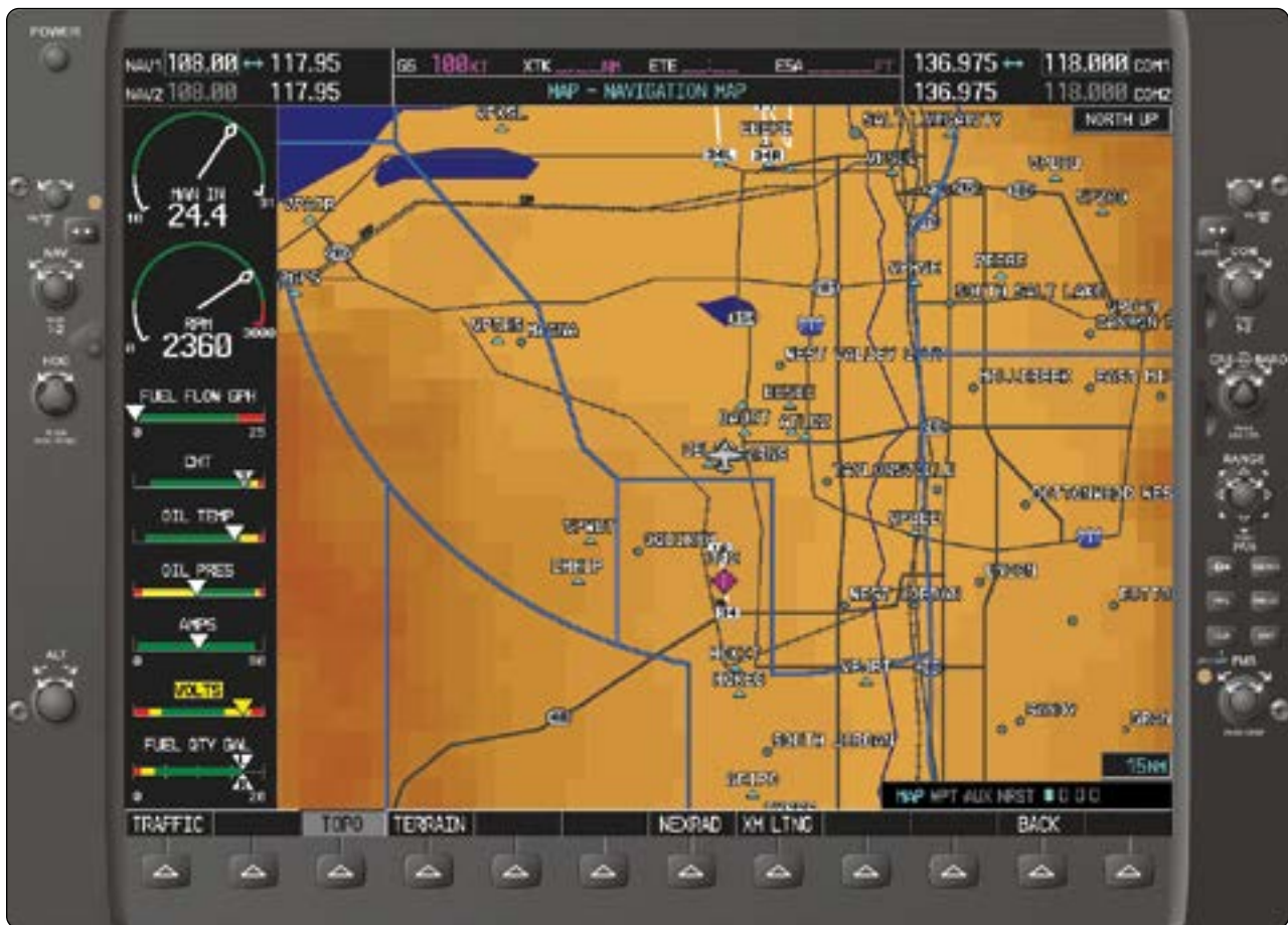
Figure 10-14. Oil pressure indication with other engine-related parameters shown in a column on the left side of this digital flight deck display panel.
