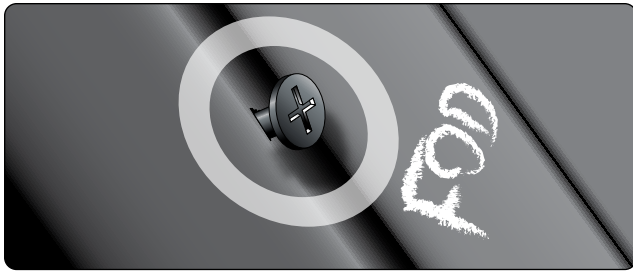
Figure 13-138. Marking of damaged area to enable closer inspection.
