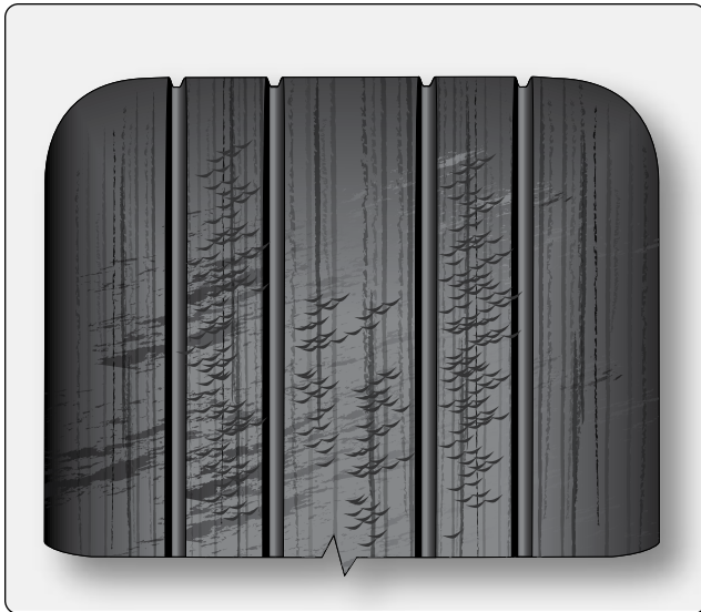
Figure 13-143. Chevron cuts in a tire are caused by operation on grooved runway surfaces. Shallow chevron cuts are permitted on aircraft tires.
