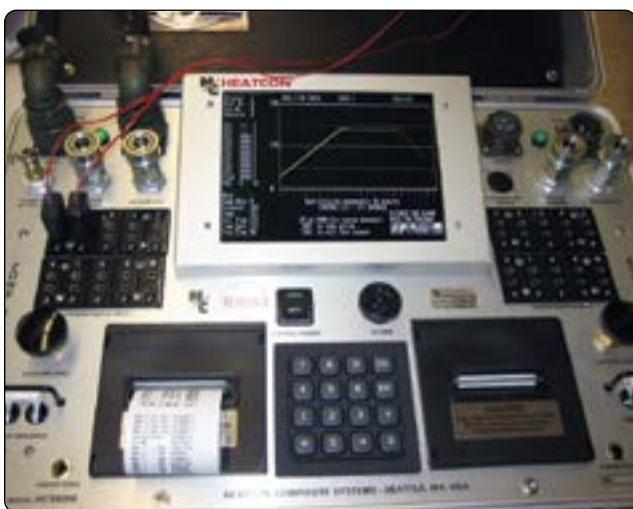
Figure 7-40. Heat bonder equipment.
