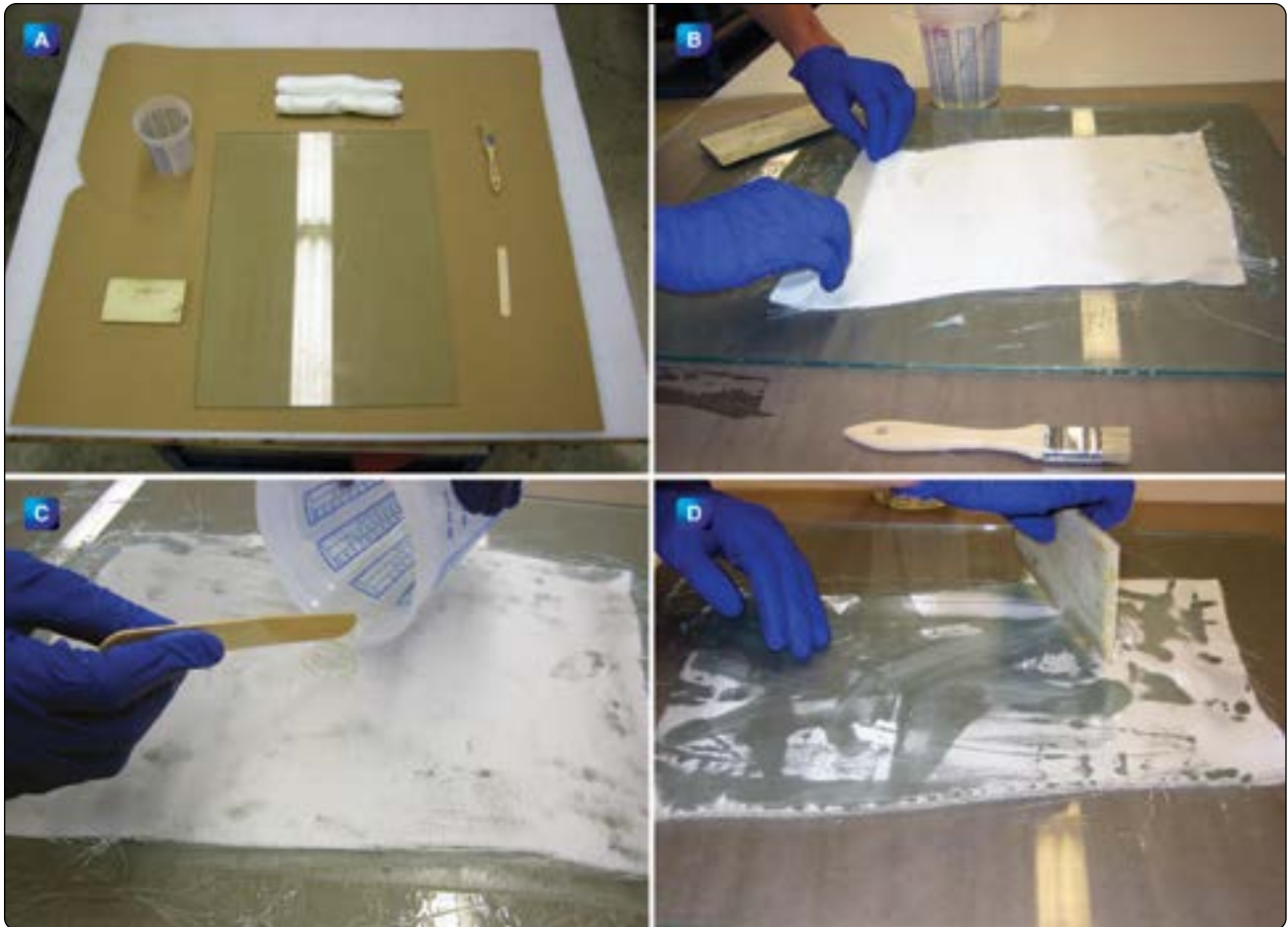
Figure 7-51. Fabric impregnation with a brush or squeegee: A) wet layup materials; B) fabric placement; C) fabric impregnation; D) squeegee used to thoroughly wet the fabric.
