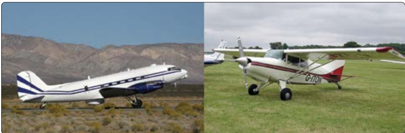
Figure 13-3. Tail wheel configuration landing gear on a DC-3 (left) and a STOL Maule MX-7-235 Super Rocket.
