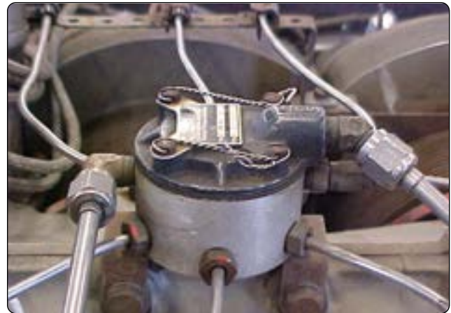
Figure 14-15. A fuel distribution manifold for a fuel-injected engine.
