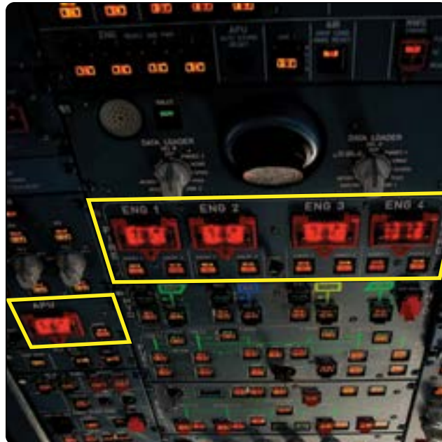
Figure 17-16. Engine and APU fire switches on the flight deck center overhead panel.
