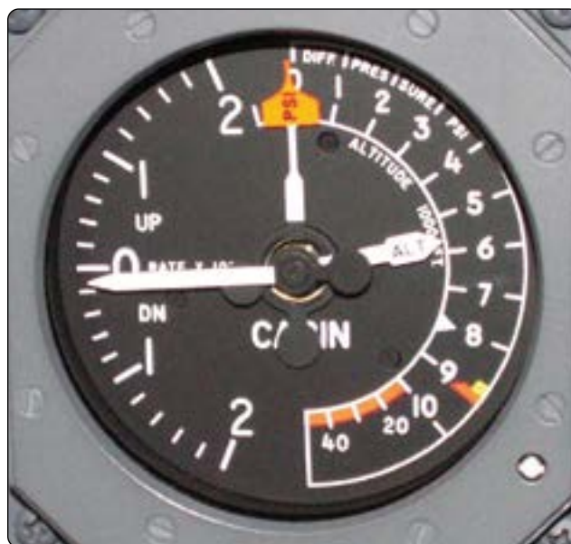
Figure 16-57. This cabin pressurization gauge is a triple combination gauge. The long pointer operates identically to a vertical speed indicator with the same familiar scale on the left side of the gauge. It indicates the rate of change of cabin pressure. The orange PSI pointer indicates the differential pressure on the right side scale. The ALT indicator uses the same scale as the PSI pointer, but it indicates cabin altitude when ALT indicator moves against it.
