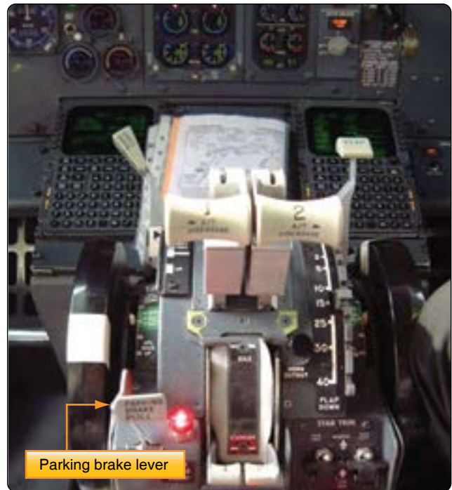
Figure 13-103. The parking brake lever on a Boeing 737 center pedestal throttle quadrant.
