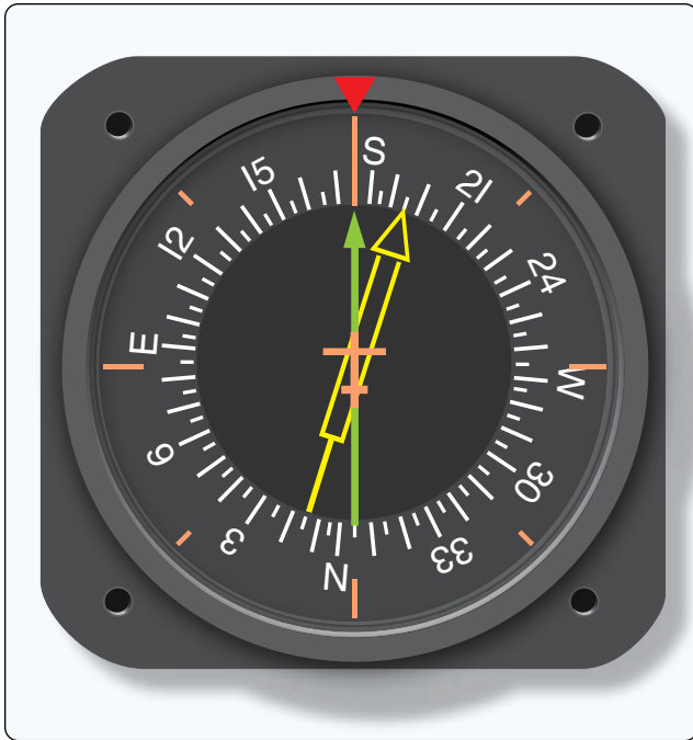
Figure 10-85. A radio magnetic indicator (RMI) combines a slaved gyro heading indication (red triangle at top of gauge) with magnetic bearing information to a VOR station (solid pointer) and an ADF station (hollow pointer).
