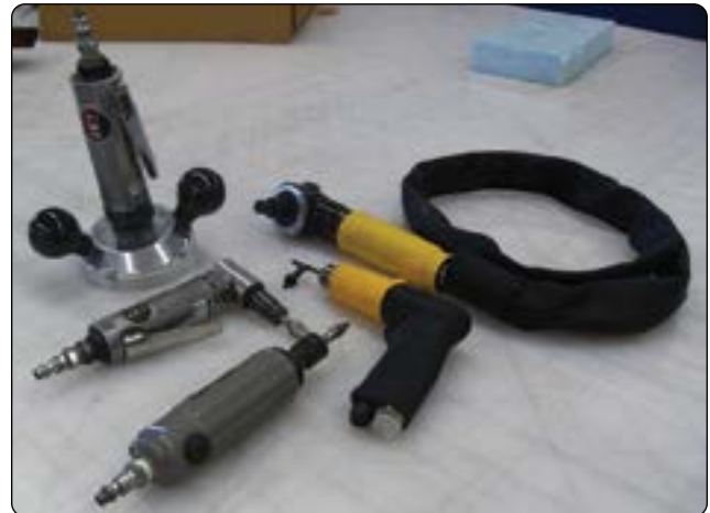
Figure 7-32. Air tools used for composite repair.
