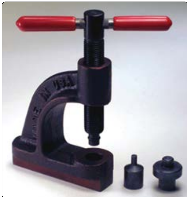
Figure 13-125. Rivet setting tool is used to install brake linings on Cleveland brake pressure plates and back plates.
