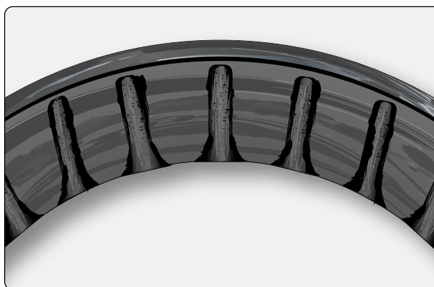
Figure 13-70. Staining and surface marks on the bearing cup that are grayish black streaks with the same spacing as the rollers are caused by water that has gotten into the bearing. It is the first stage of deeper corrosion that will follow.
