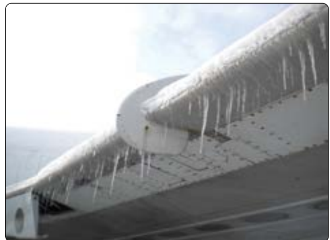
Figure 15-1. Formation of ice on aircraft leading edge.
