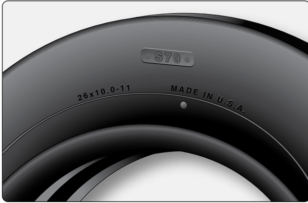
Figure 13-133. A sidewall vent marked by a colored dot must be kept free from obstruction to allow trapped air or nitrogen to escape from the carcass plies of the tire.
