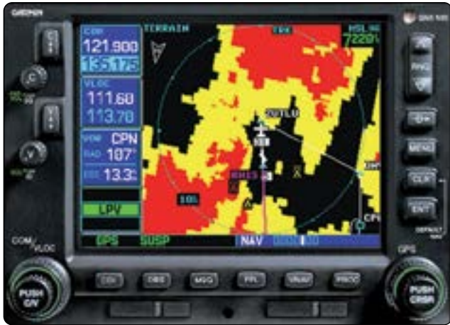
Figure 11-153. A GPS unit integrated with NAV/COM circuitry.
