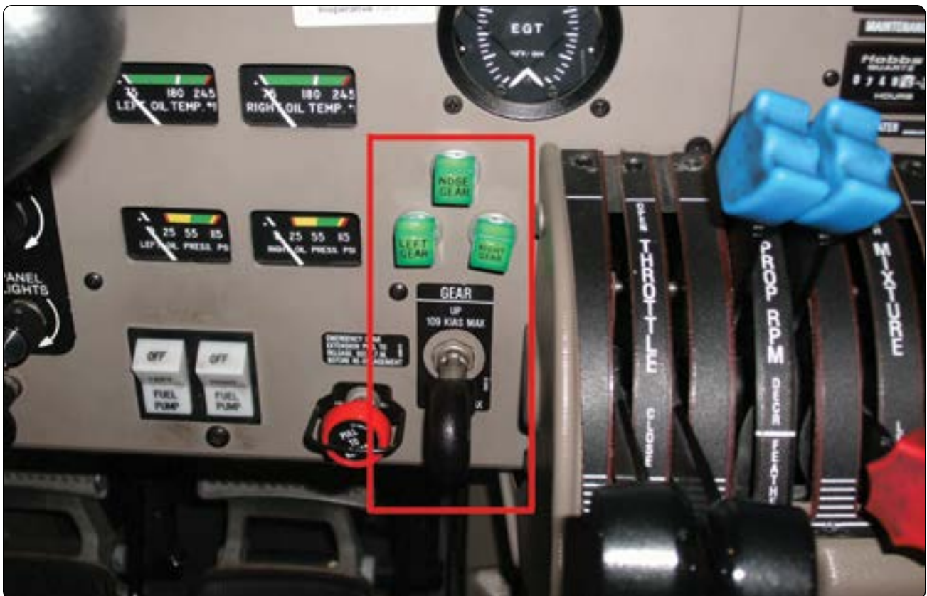
Figure 9-94. Instrument panel showing the landing gear position switch and the three gear down indicators.
