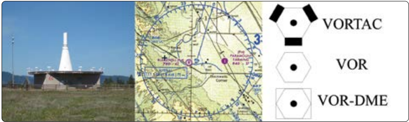
Figure 11-95. A VOR ground station.
