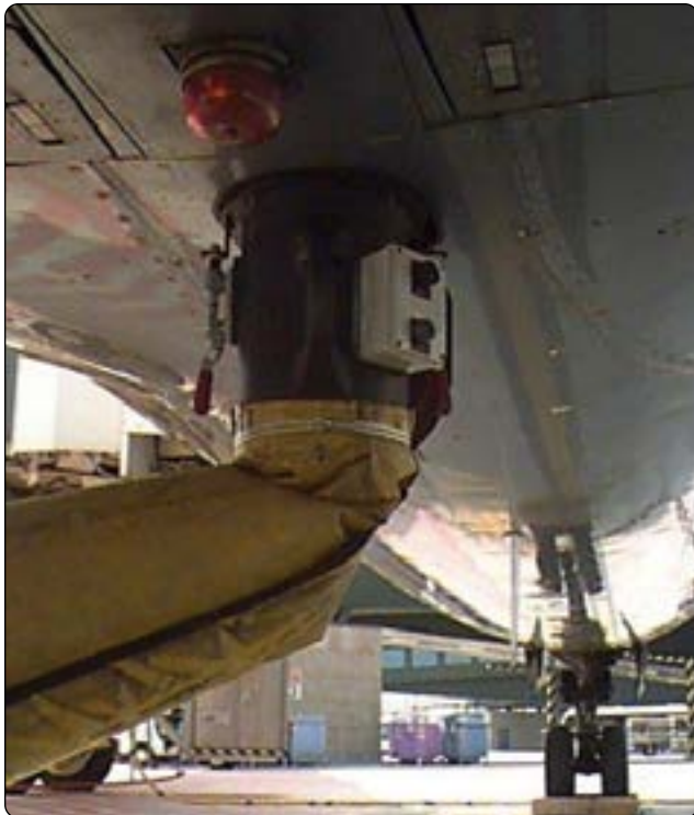
Figure 16-61. A duct hose installed on this airliner distributes hot or cold air from a ground-based source throughout the cabin using the aircraft's own air distribution system ducting.
