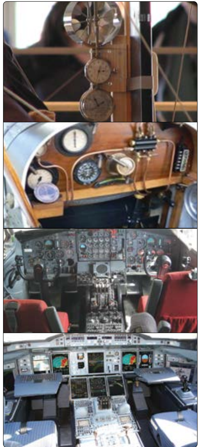
Figure 10-1. From top to bottom: instruments of the Wright Flyer, instruments on a World War I era aircraft, a late 1950s/early 1960s Boeing 707 airliner flight deck, and an Airbus A380 glass flight deck.
