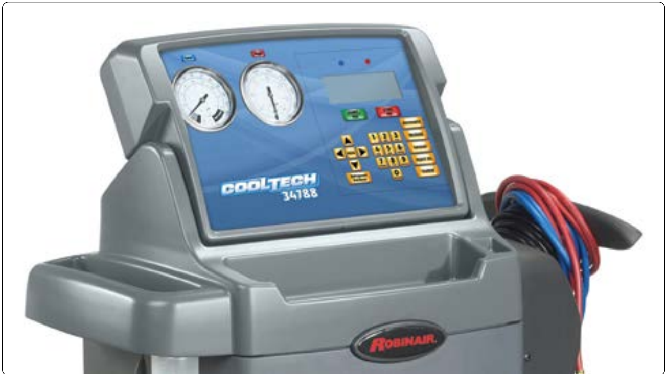
Figure 16-88. A modern refrigerant recovery/recycle/charging service unit. Electronic control of solenoid activated valves combine with a built-in system for recovering, recycling, and recharging. A built-in vacuum pump and heated refrigerant reservoir are also included.
