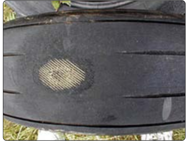
Figure 13-141. Landing with the brake on causes a tire flat spot that exposes the under tread and requires replacement of the tire.
