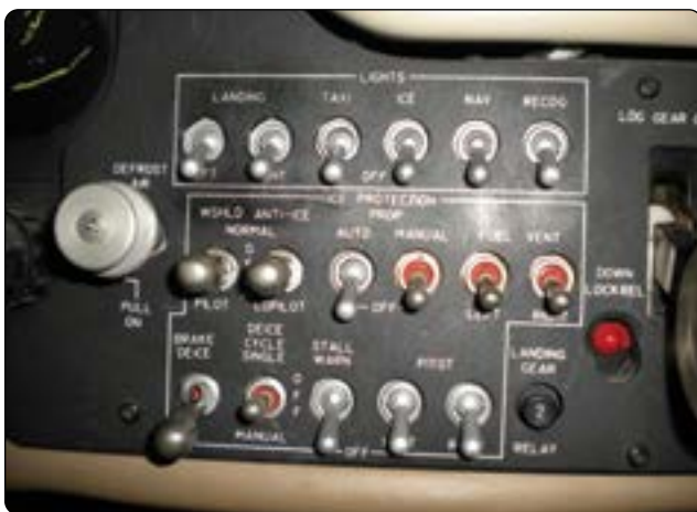
Figure 15-22. Ice protection panel on a turboprop aircraft with deice boots.
