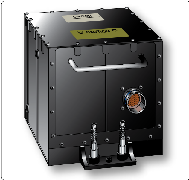
Figure 11-156. A modern micro-IRS with built-in GPS.
