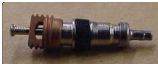
Figure 13-149. The tire valve core should be removed after the tire is completely deflated and before the tire and wheel assembly is removed from the aircraft.
