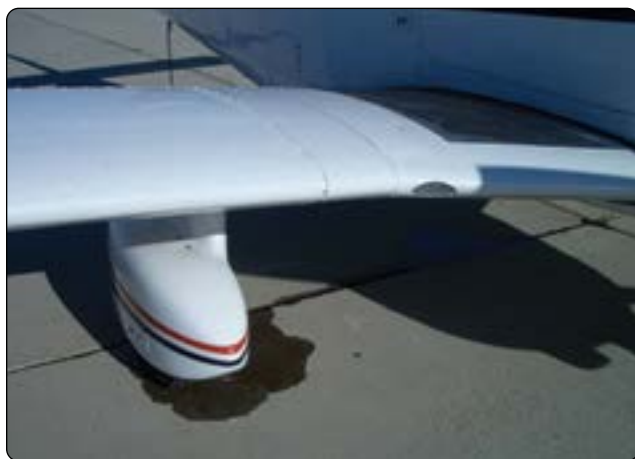
Figure 13-121. The cause of all aircraft brake leaks must be investigated, repaired, and tested before releasing the aircraft for flight.
