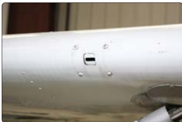
Figure 10-61. A reed-type stall warning device is located behind this opening in the leading edge of the wing. When the angle of attack increases to near the point of a stall, low-pressure air flowing over the opening causes a suction, which audibly vibrates the reed.
