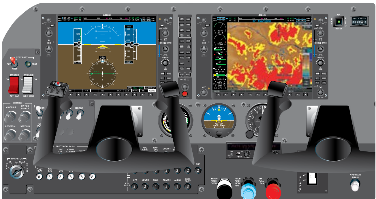
Figure 10-99. Instrumentation displayed within a glass flight deck using an attitude heading and reference system (AHRS) computer.
