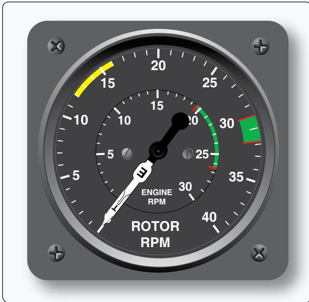
Figure 10-57. A helicopter tachometer with engine rpm, rotor rpm, and slippage indications.
