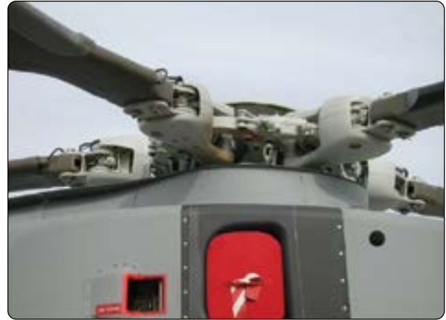
Figure 1-99. Five-blade articulated main rotor with elastomeric bearings.
