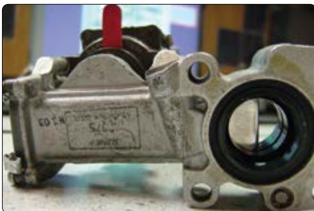
Figure 14-40. This motor-operated gate valve has a red position indicating lever that can be used by maintenance personnel to identify the position of the valve. The lever can be moved by the technician to position the valve.
