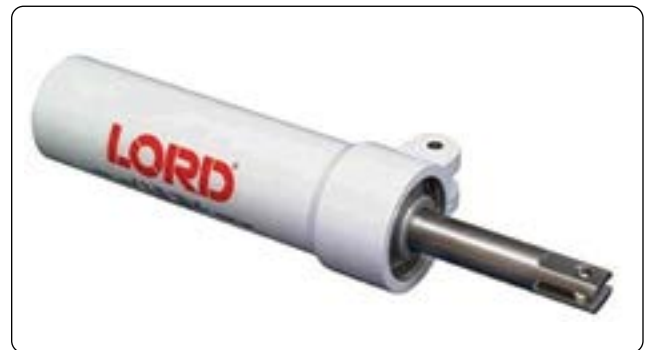
Figure 13-57. A non-hydraulic shimmy damper uses a rubber piston with lubricant that dampens via motion against the inner diameter of the unit housing.
