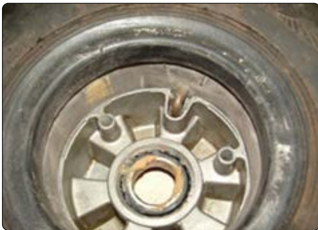
Figure 13-158. Mounting a tube type tire with the tube valve stem positioned to pass through the outboard wheel half.
