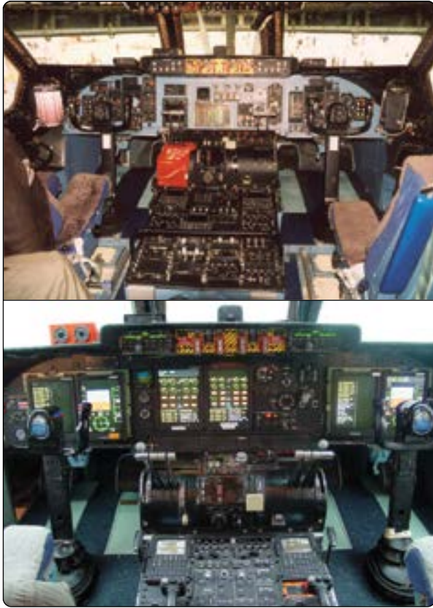
Figure 10-2. A conventional instrument panel of the C-5A Galaxy (top) and the glass flight deck of the C-5B Galaxy (bottom).
