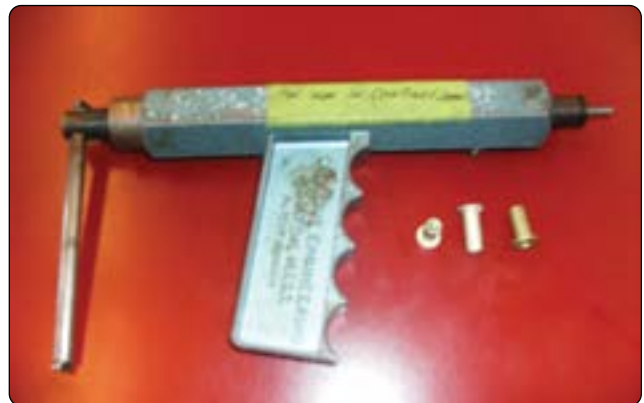
Figure 4-113. Rivet nut installation.
