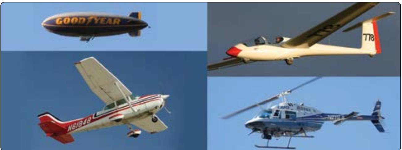
Figure 1-11. Examples of different categories of aircraft, clockwise from top left: lighter-than-air, glider, rotorcraft, and airplane.
