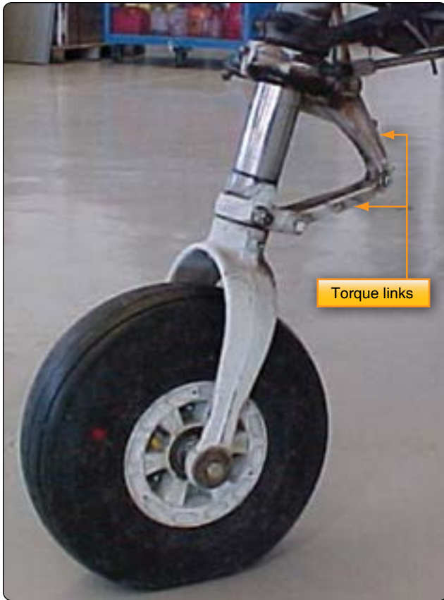
Figure 13-19. Torque links align the landing gear and retain the piston in the upper cylinder when the strut is extended.
