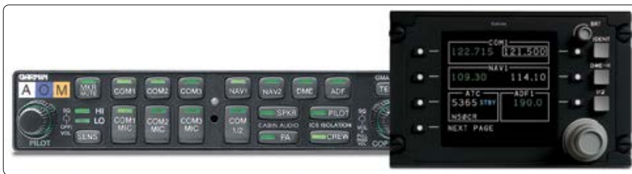
Figure 11-73. An audio panel in a general aviation aircraft integrates the selection of several radio-based communication and navigational aids into a single control panel (left). A digital tuner (right) does the same on a business class aircraft and allows the frequency of each device to be tuned from the same panel as well.
