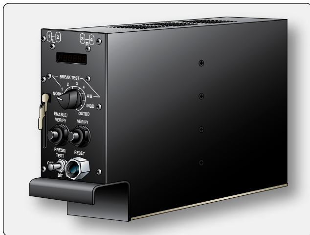
Figure 13-109. A rack mounted anti-skid control unit from an airliner.
