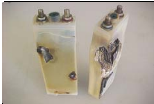
Figure 9-35. Thermal runaway damage.
