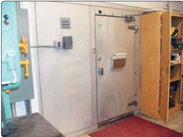
Figure 7-44. Walk-in freezer for storing prepreg materials.
