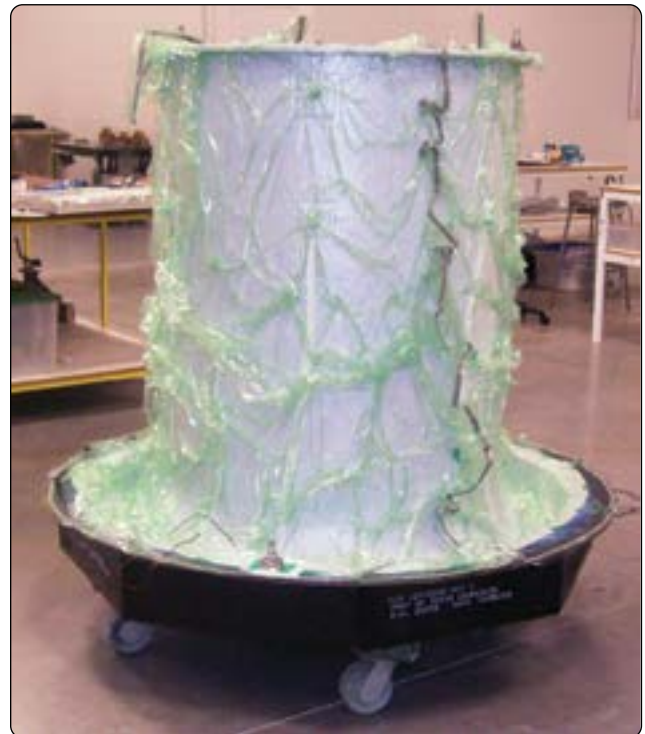
Figure 7-36. Bagging of complex part.
