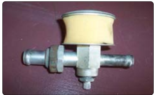
Figure 10-89. A vacuum regulator, also known as a suction relief valve, includes a foam filter. To relieve vacuum, outside air of a higher pressure must be drawn into the system. This air must be clean to prevent damage to the pump.
