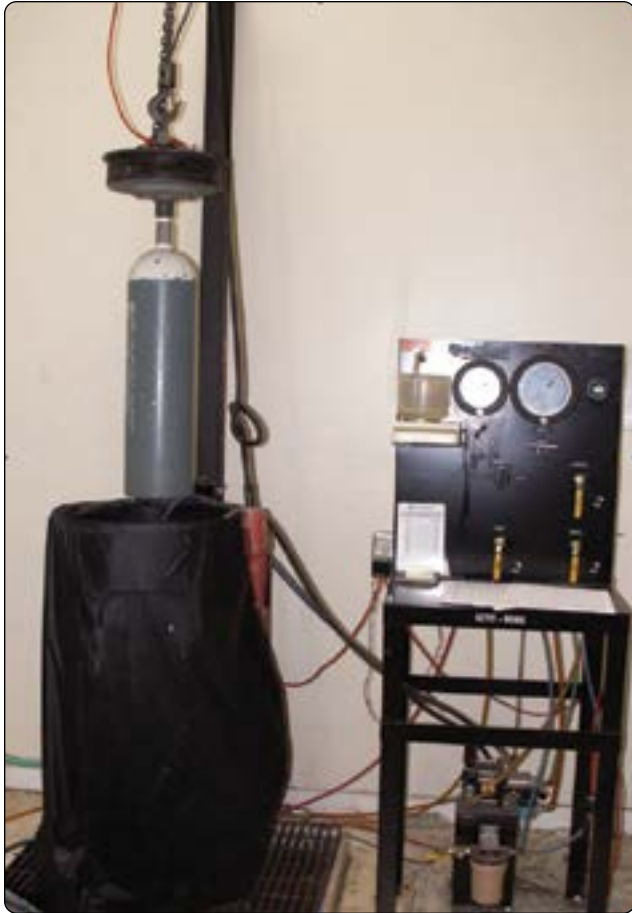
Figure 16-9. This test stand is used for hydrostatic testing of oxygen cylinders. The water-filled cylinder is lowered into the barrel on the left where it is pressurized to the proper level as monitored via gauges mounted on the control panel. A displacement container on the top left of the control board collects water from the barrel to measure the expansion of the cylinder when pressurized to ensure it is within limits.
