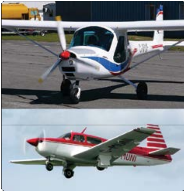
Figure 1-87. Tricycle landing gear is the most predominant landing gear configuration in aviation.
