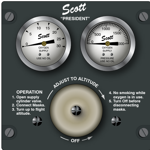
Figure 16-12. A manual continuous flow oxygen system may have a regulator that is adjusted by the pilot as altitude varies. By turning the knob, the left gauge can be made to match the flight altitude thus increasing and decreasing flow as altitude changes.
