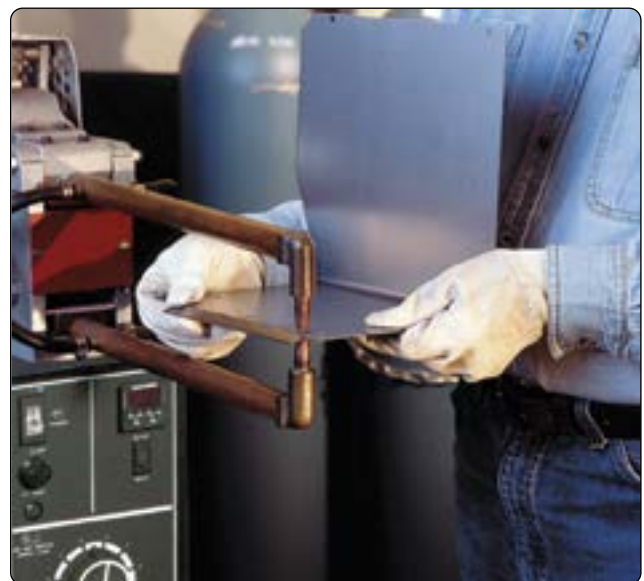
Figure 5-10. Spot welding thin sheet metal.
