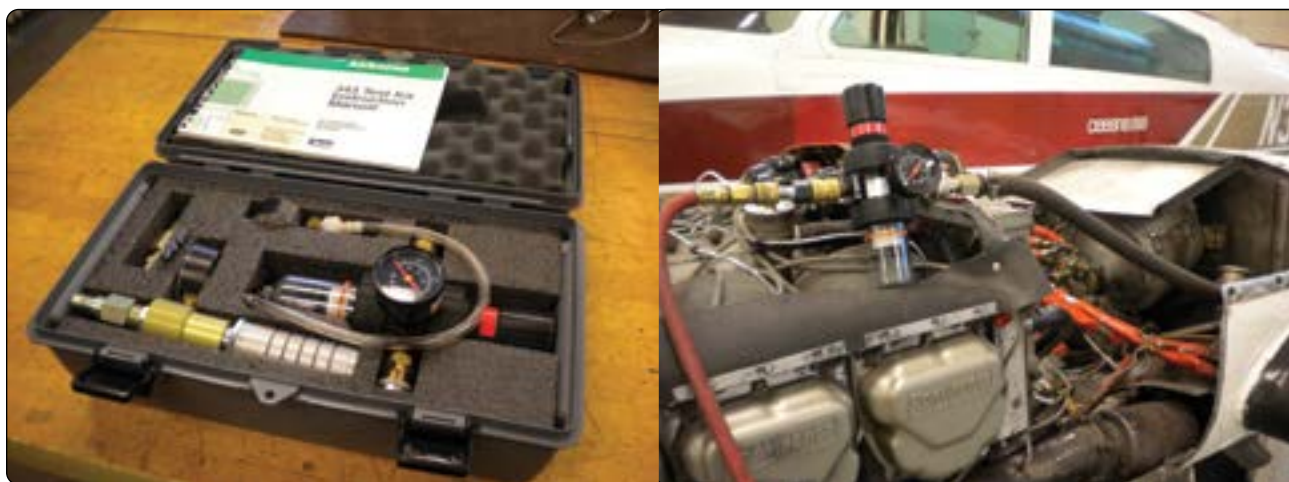
Figure 15-32. Test equipment used to test a wing deice system (left), and test equipment installed in the aircraft for testing (right).
