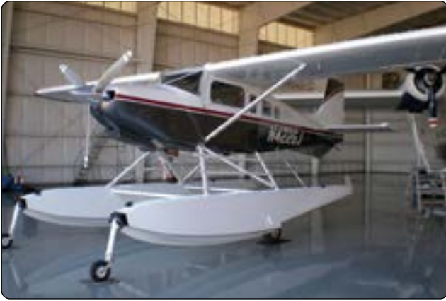
Figure 1-85. Retractable wheels make this aircraft amphibious.
