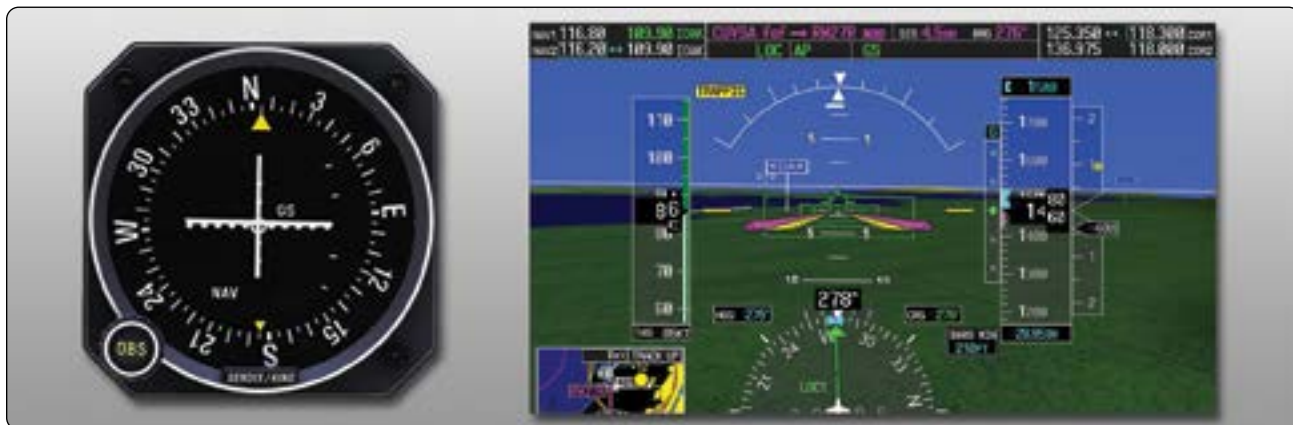
Figure 11-113. A traditional course deviation indicator is shown on the left. The horizontal white line is the deviation indicator for the glideslope. The vertical line is for the localizer. On the right, a Garmin G-1000 PFD illustrates an aircraft during an ILS approach. The narrow vertical scale on the right of the attitude indicator with the “G” at the top is the deviation scale for the glideslope. The green diamond moves up and down to reflect the aircraft being above or below the glidepath. The diamond is shown centered indicating the aircraft is on course vertically. The localizer CDI can be seen at the bottom center of the display. It is the center section of the vertical green course indicator. LOC1 is displayed to the left of it.
