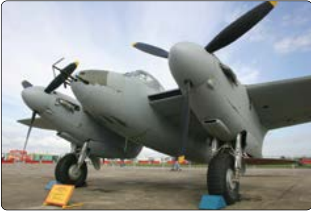
Figure 1-9. The De Havilland Mosquito used a laminated wood construction with a balsa wood core in the fuselage.
