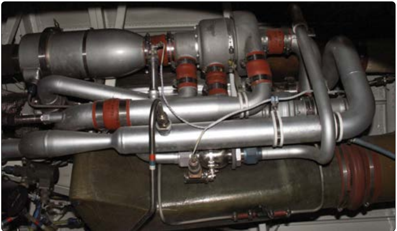
Figure 16-50. An air cycle air conditioning system used to pressurize the cabin of a business jet.
