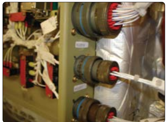
Figure 9-161. Connector arrangement to avoid wrong connection.
