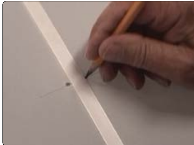
Figure 3-25. A premarked location for a lacing hole, which is punched through the fabric with a pencil.
