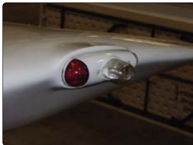
Figure 9-174. A left wing tip position light (red) and a white strobe light.
