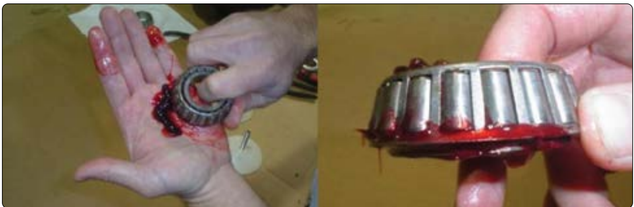
Figure 13-46. Packing grease into a clean, dry bearing can be done by hand in the absence of a bearing grease tool. Press the bearing into the grease on the palm of the hand until it passes completely through the gap between the rollers and the inner race all the way around the bearing.
