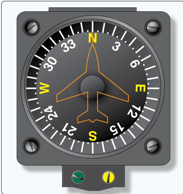
Figure 10-81. A vertical magnetic direction indicator provides a realistic reference of headings.
