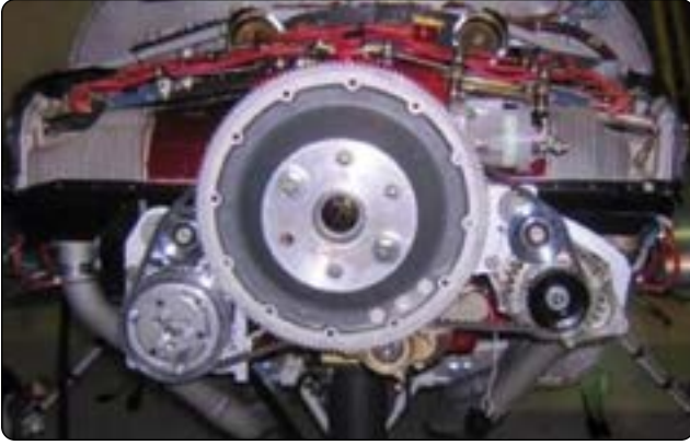
Figure 16-81. A typical belt drive engine driven compressor. The electromagnetic clutch pulley assembly in the front starts and stops the compressor depending on cooling demand.
