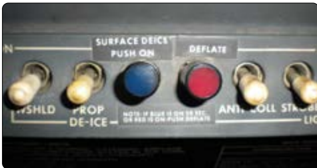
Figure 15-19. Wing deice switch.
