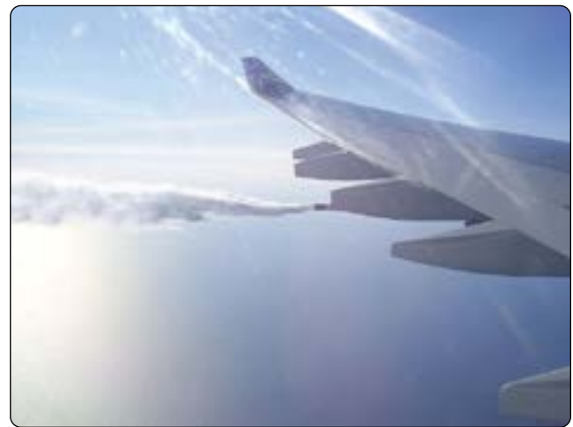
Figure 14-3. Fuel being jettisoned free of the airframe on a transport category aircraft.
