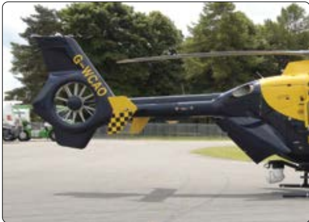
Figure 1-101. A Fenestron or “fan-in-tail” antitorque system. This design provides an improved margin of safety during ground operations.
