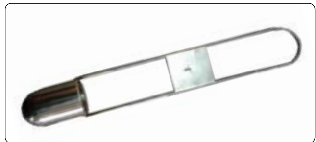
Figure 8-10. A Zahn cup viscosity measuring cup.
