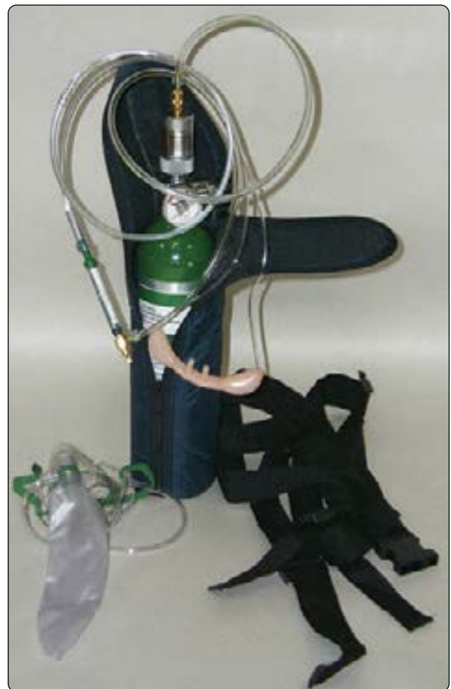
Figure 16-11. A typical portable gaseous oxygen cylinder complete with valve, pressure gauge, regulator/reducer, hose, adjustable flow indicator, and rebreather cannula. A padded carrying case/bag can be strapped to the back of a seat in the cabin to meet certification and testing specifications.
