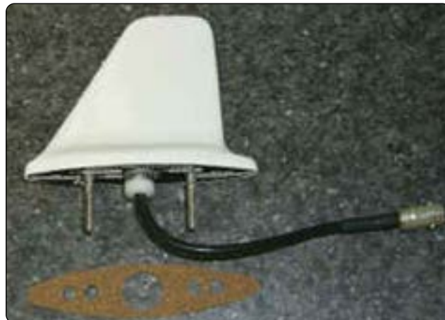
Figure 11-121. A typical aircraft-mounted DME antenna.
