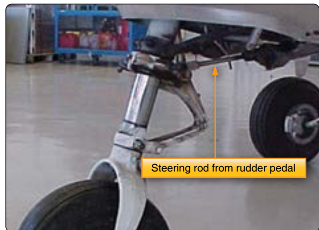
Figure 13-51. Nose wheel steering on a light aircraft often uses a push-pull rod system connected to the rudder pedals.
