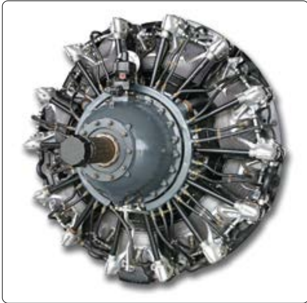
Figure 16-43. The radial engine supercharger cannot be used since fuel is introduced before the supercharger impeller compresses the air.
