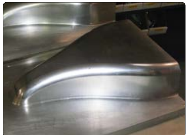
Figure 7-34. A mold of an inlet duct.
