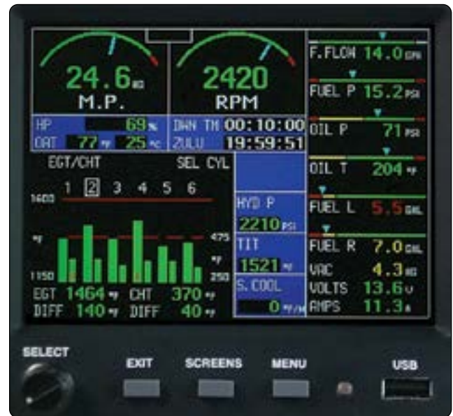
Figure 11-72. A digital data display dedicated to the depiction of engine and airframe system parameter status.
