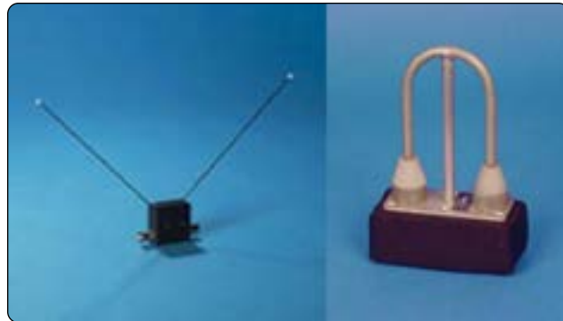
Figure 11-114. Glideslope antennas—designed to be mounted inside a non-metallic aircraft nose (left), and mounted inside or outside the aircraft (right).
