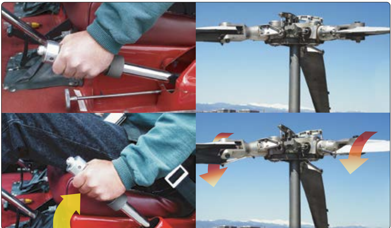
Figure 2-45. Raising the collective pitch control increases the pitch angle by the same amount on all blades.
