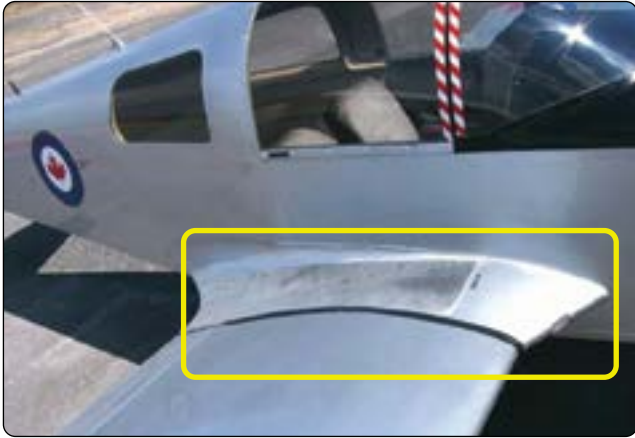
Figure 1-33. Wing root fairings smooth airflow and hide wing attach fittings.
