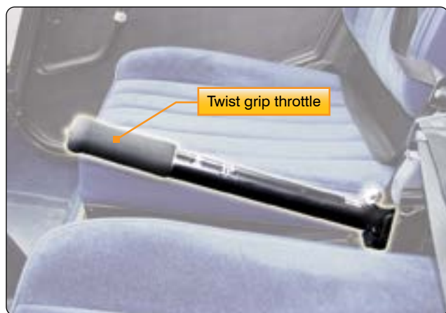
Figure 2-46. A twist grip throttle is usually mounted on the end of the collective lever. The throttles on some turbine helicopters are mounted on the overhead panel or on the floor in the flight deck.
