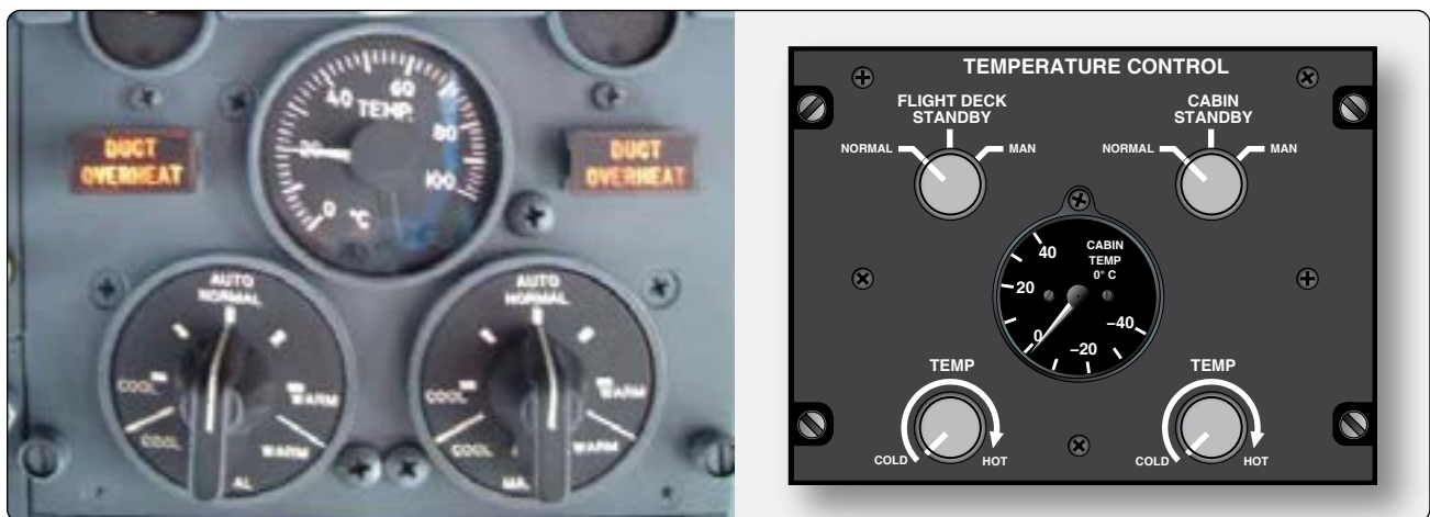
Figure 16-70. Typical temperature selectors on a transport category aircraft temperature control panel in the flight deck (left) and a business jet (right). On large aircraft, temperature selectors may be located on control panels located in a particular cabin air distribution zone.
