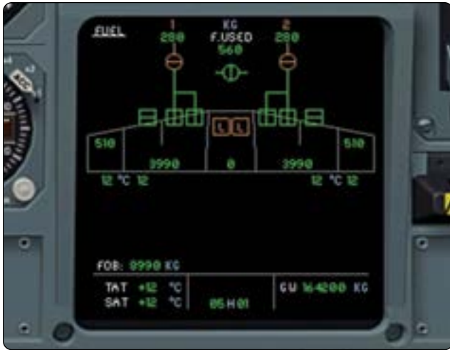
Figure 14-39. The graphic depiction of the fuel system on this electronic centralized aircraft monitor (ECAM) fuel page includes valve position information.
