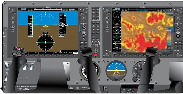
Figure 10-5. This electrically operated flat screen display instrument panel, or glass flight deck, retains an analog airspeed indicator, a gyroscope-driven artificial horizon, and an analog altimeter as a backup should electric power be lost, or a display unit fails.
