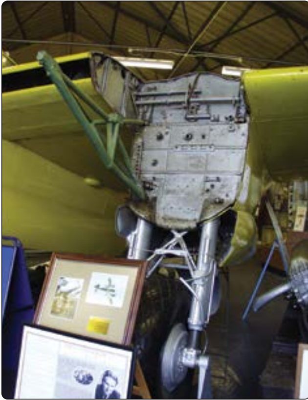
Figure 1-41. An engine nacelle firewall.
