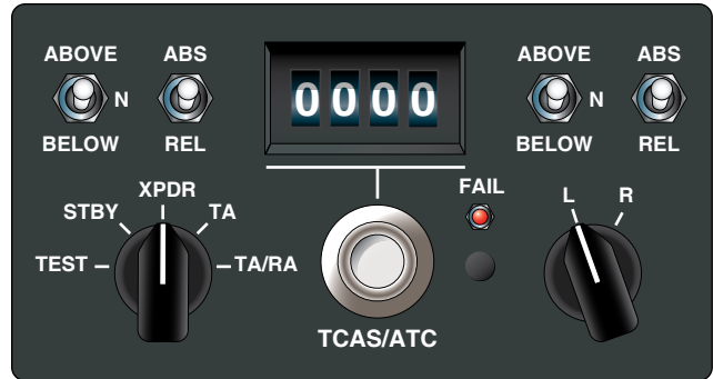
Figure 11-134. This control panel from a Boeing 767 controls the transponder for ATC use and TCAS.
