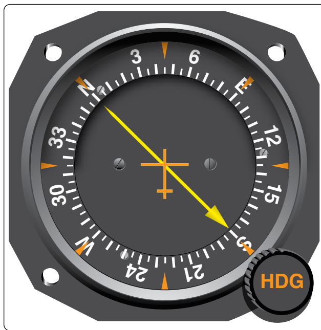
Figure 11-104. A movable card ADF indicator can be rotated to put the aircraft's heading at the top of the scale. The pointer then points to the magnetic bearing the ADF broadcast antenna.
