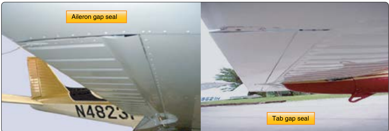
Figure 1-81. Gap seals promote the smooth flow of air over gaps between fixed and movable surfaces.
