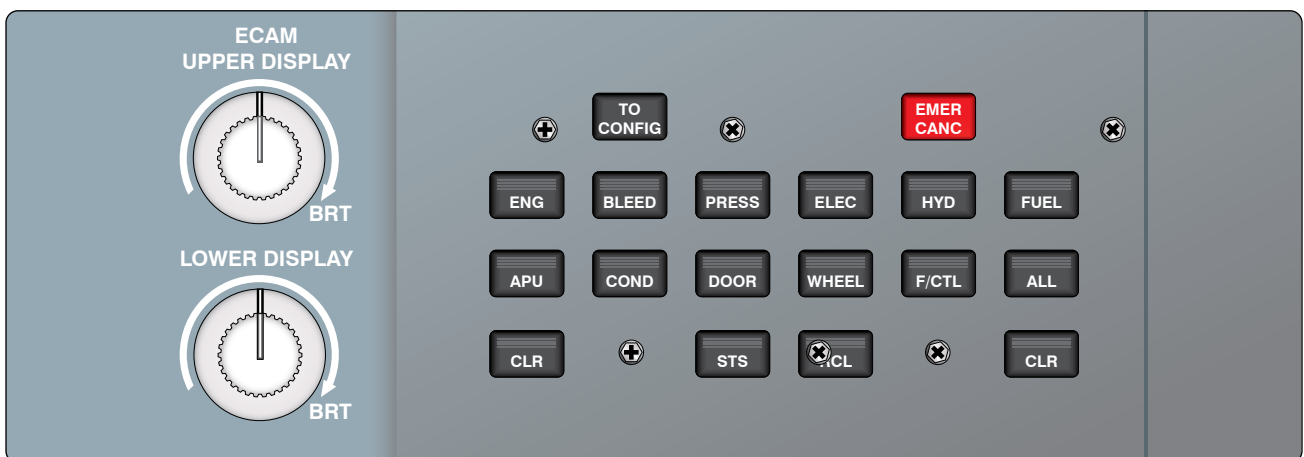
Figure 10-121. An ECAM display control panel.
