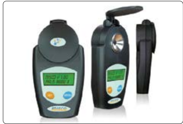
Figure 14-94. A hand-held refractometer with digital display measures the amount of fuel anti-ice additive contained in a fuel load.
