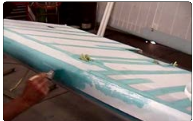
Figure 3-34. Cement is brushed through a four-inch tape during installation over the fabric seam on a wing leading edge. Two-inch tapes cover the wing ribs and rib lacing.
