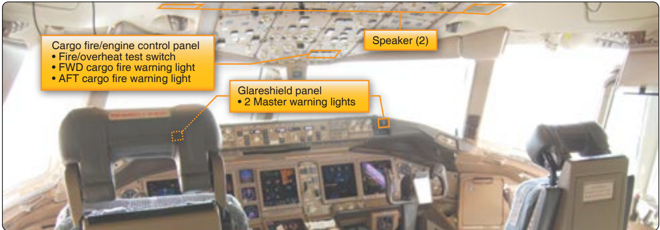
Figure 17-18. Cargo fire detection warning.
