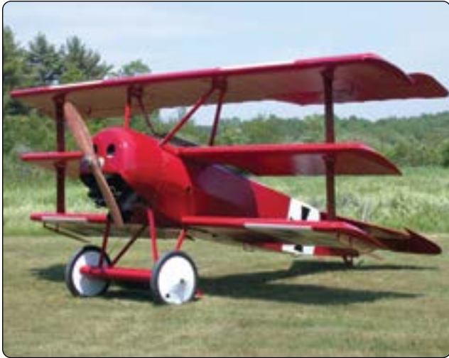
Figure 13-14. Rigid steel landing gear is used on many early aircraft.
