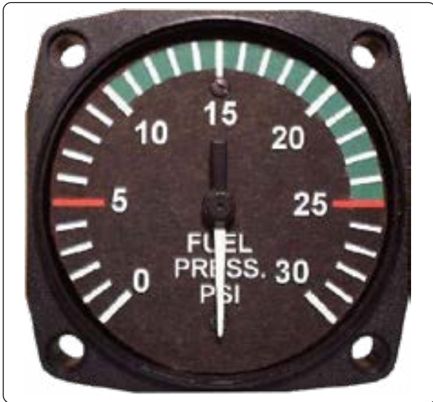
Figure 10-17. A typical analog fuel pressure gauge.
