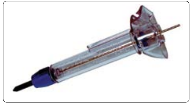
Figure 14-93. A sump drain tool used to open and collect fuel and contaminants from the fuel system sumps. Daily sump draining is part of the procedures needed to remove water from fuel that is to be delivered to the engine(s).
