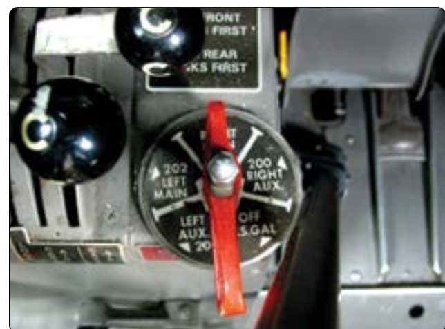
Figure 14-38. Detents for each position, an indicating handle, and labeling aid the pilot in knowing the position of the fuel valve.
