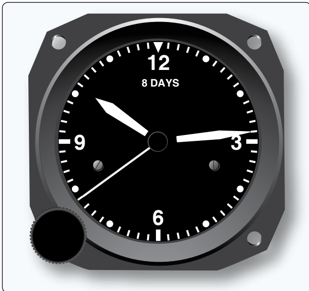
Figure 10-131. A typical mechanical 8-day aircraft clock.
