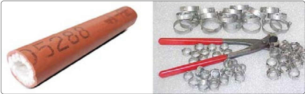
Figure 14-36. Exterior fuel hose wrap that protects from fire, as well as abrasion, shown with the clamps and pliers used to install it.
