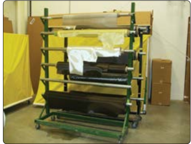
Figure 7-12. Dry fabric materials (top to bottom: aluminum lightning protection mesh, Kevlar®, fiberglass, and carbon fiber).
