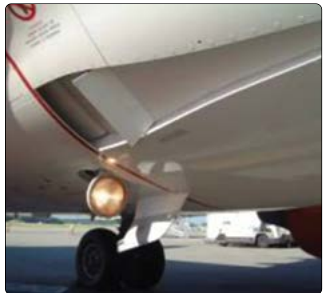
Figure 16-66. A ram air door controls the flow of air through the primary and secondary heat exchangers.
