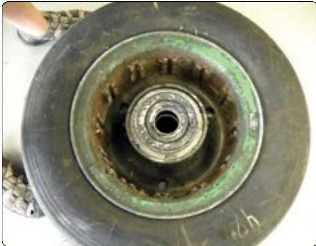
Figure 13-61. Keys on the inner wheel half of an aircraft wheel used to engage and rotate the rotors of a disc brake.
