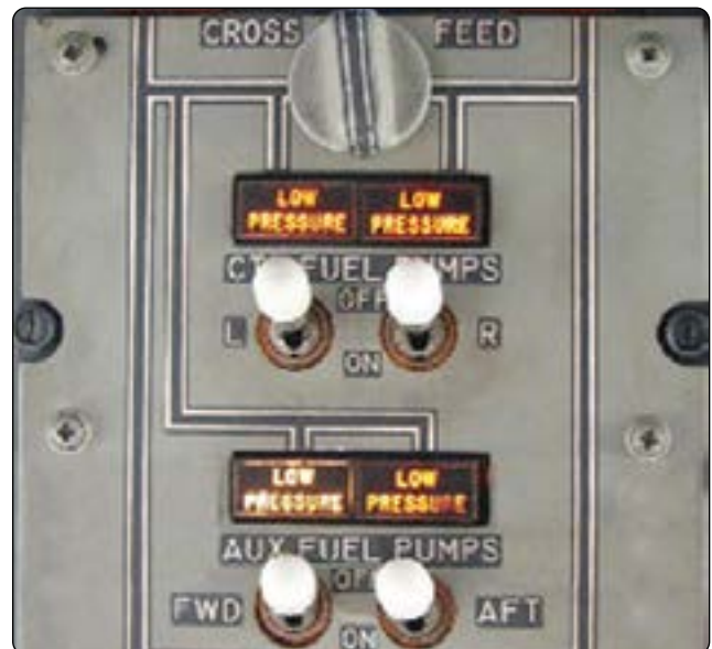
Figure 14-87. A transport category aircraft fuel panel with low pressure warning lights for each fuel boost pump.
