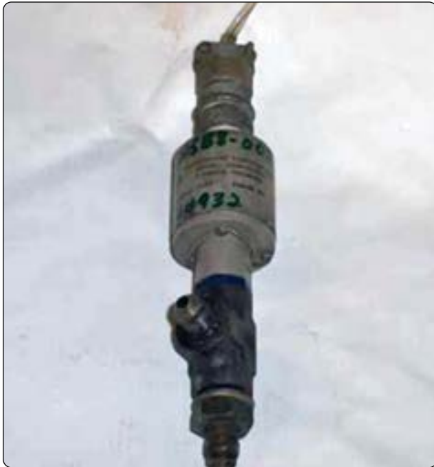
Figure 10-20. A pressure switch can be used in addition to, or instead of, a pressure gauge.
