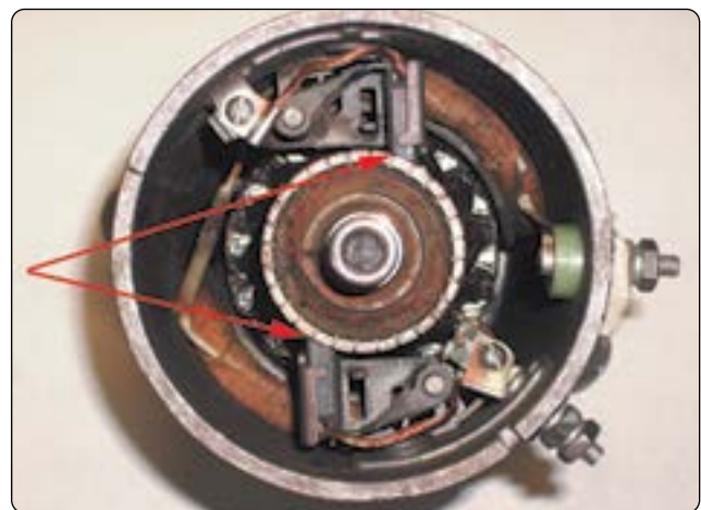
Figure 9-52. Wear areas of commutator and brushes.
