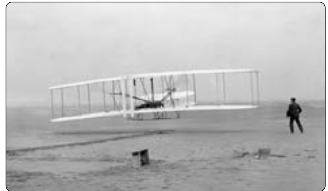
Figure 1-4. The Wright Flyer was the first successful powered aircraft. It was made primarily of wood and fabric.
