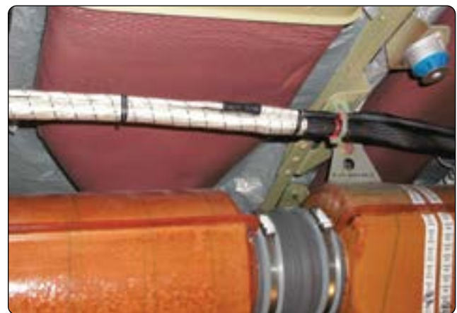
Figure 9-113. Shielded wire harness for flight control.
