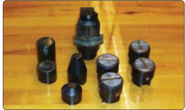
Figure 4-66. Shrinking and stretching tools.
