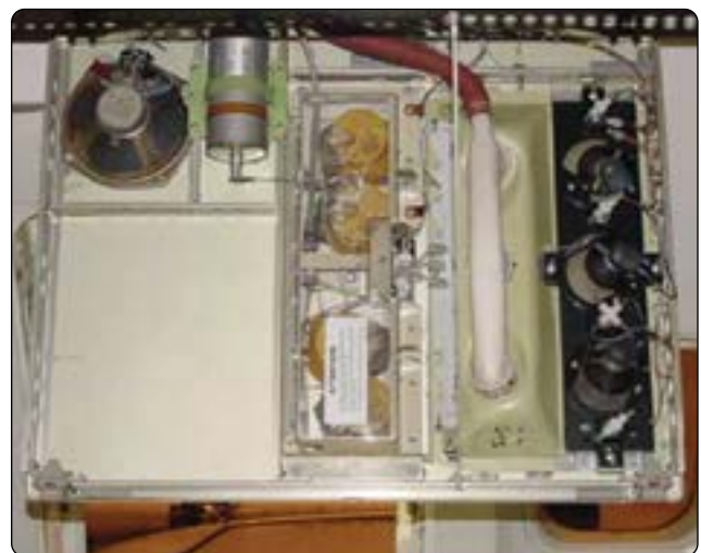
Figure 16-29. An oxygen generator mounted in place in an overhead passenger service unit of an air transport category aircraft.
