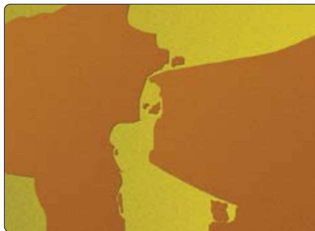
Figure 8-13. Example of poor adhesion.
