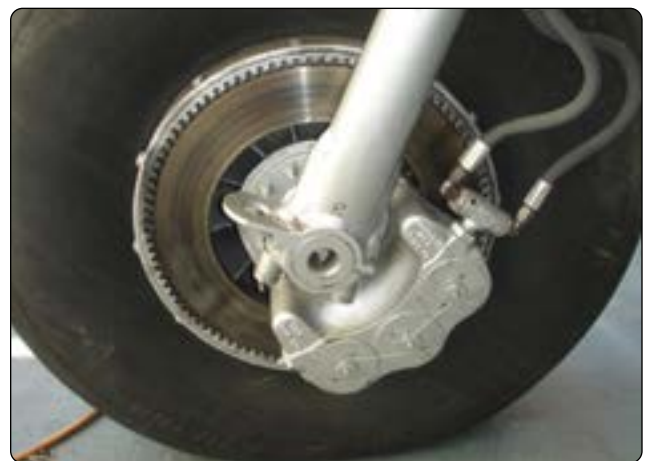
Figure 13-79. A single disc brake is a floating-disc, fixed caliper brake.
