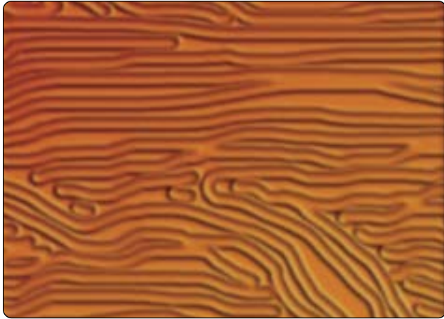
Figure 8-20. Example of wrinkling.
