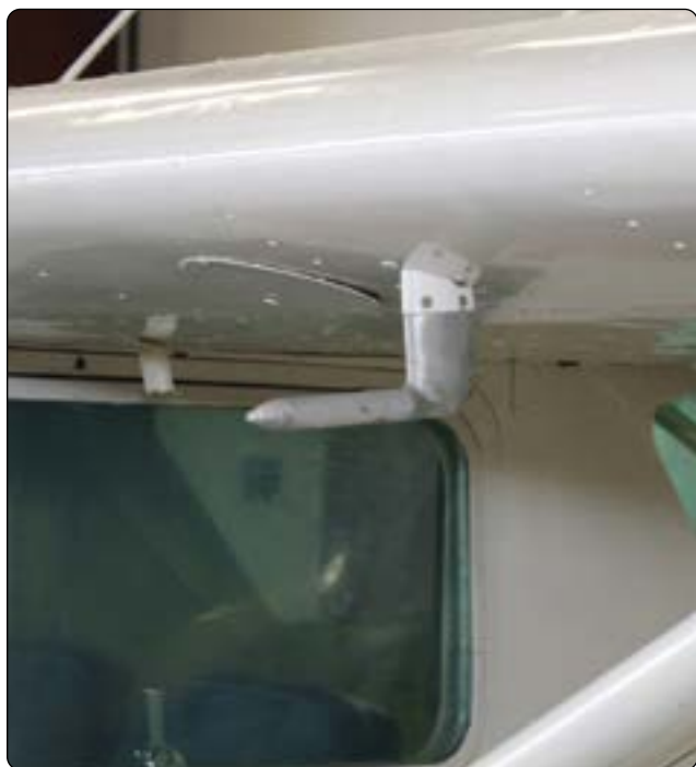
Figure 10-24. Pitot-static system heads, or pitot tubes, can be of various designs and locations on airframes.
