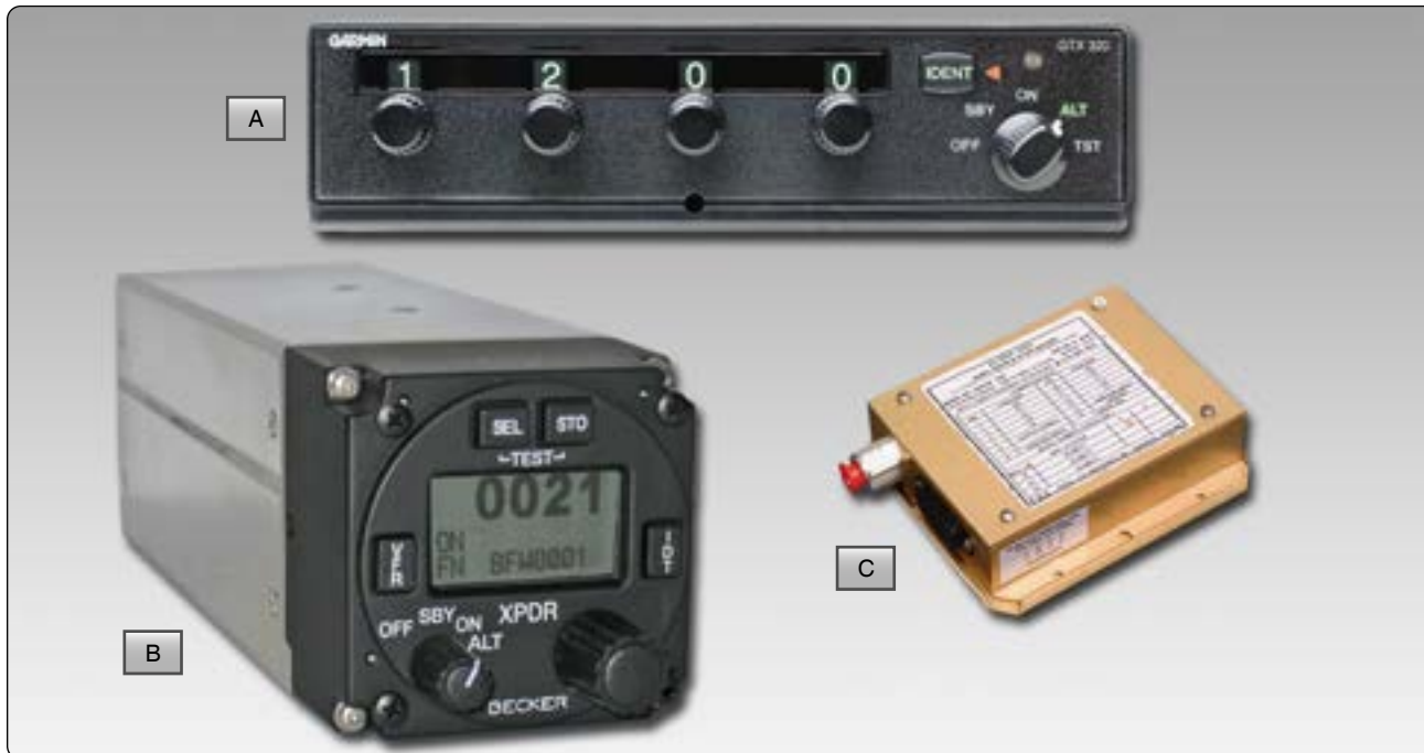
Figure 11-125. A traditional transponder control head (A), a lightweight digital transponder (B), and a remote altitude encoder (C) that connects to a transponder to provide ATC with an aircraft's altitude displayed on a PPI radar screen next to the target that represents the aircraft.
