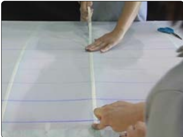
Figure 3-24. Reinforcing tape the same width as the wing ribs is applied over all wing ribs.
