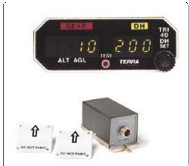
Figure 11-140. A digital display radio altimeter (top), and the two antennas and transceiver for a radio/radar altimeter (bottom).
