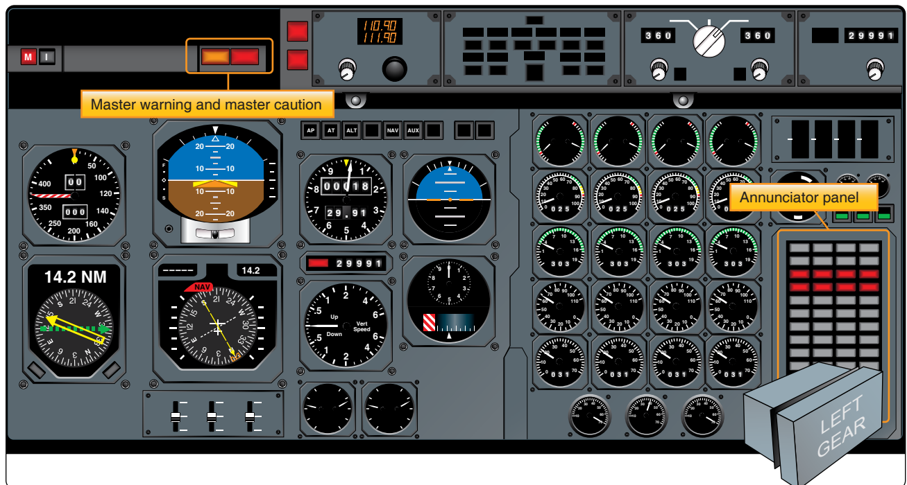
Figure 10-128. The centralized analog annunciator panel has indicator lights from systems and components throughout the aircraft. It is supported by the master caution system.
