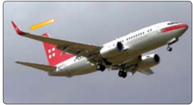
Figure 1-77. A winglet reduces aerodynamic drag caused by air spilling off of the wing tip.
