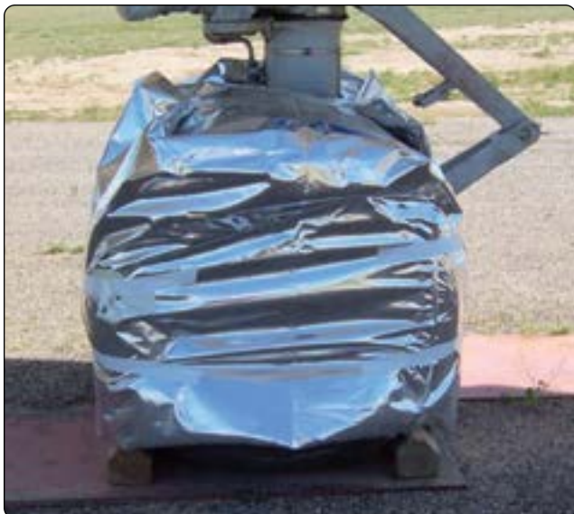
Figure 13-146. Cover tires to protect from harmful chemicals and from the elements when parked outside for long periods of time.
