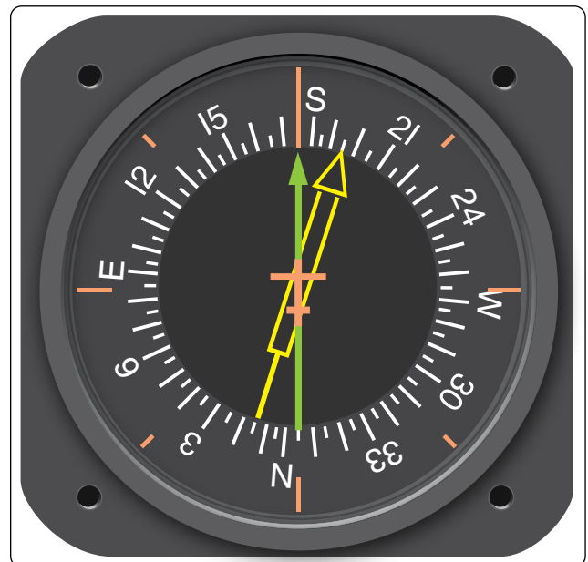
Figure 11-109. A radio magnetic indicator (RMI) combines a magnetic compass, VOR, and ADF indications.
