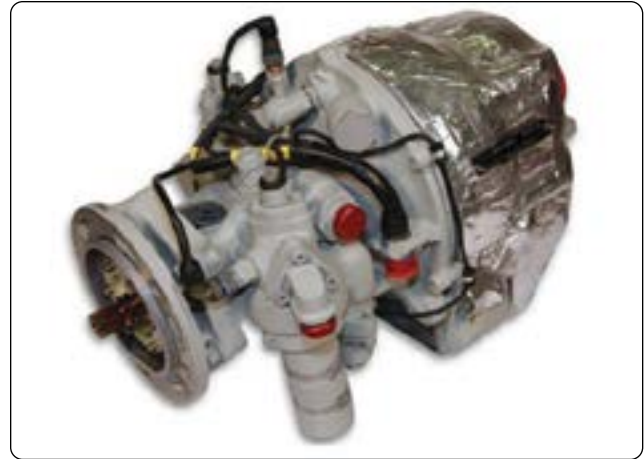
Figure 12-5. Hydraulic power pack.
