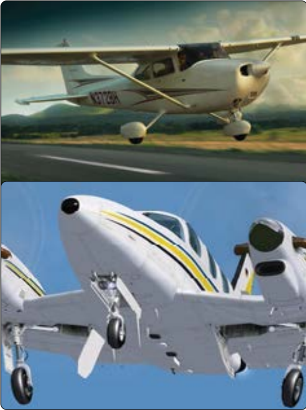
Figure 1-82. Landing gear can be fixed (top) or retractable (bottom).
