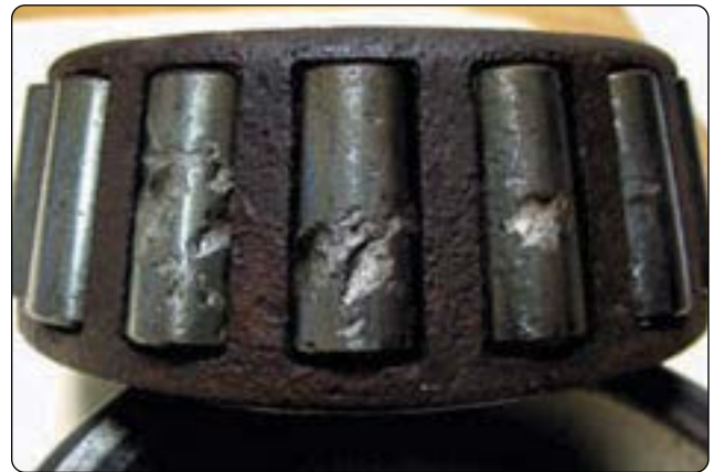
Figure 13-66. Spalling is a chipped away portion of the hardened surface of a bearing roller or race.
