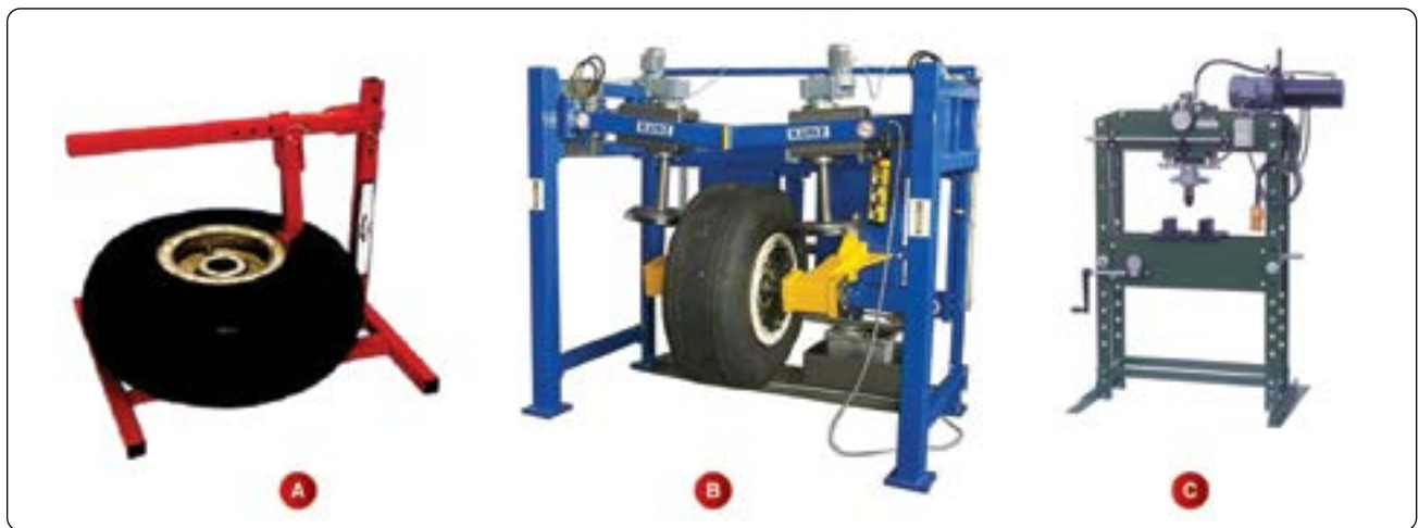
Figure 13-64. Tire beads must be broken from the wheel to remove the tire. A mechanical removal tool designed for breaking the bead is shown in (A); a hydraulic press designed with the capacity for large aircraft wheels is shown in (B); and an arbor press is shown in (C). All are tools available to the technician for this purpose.
