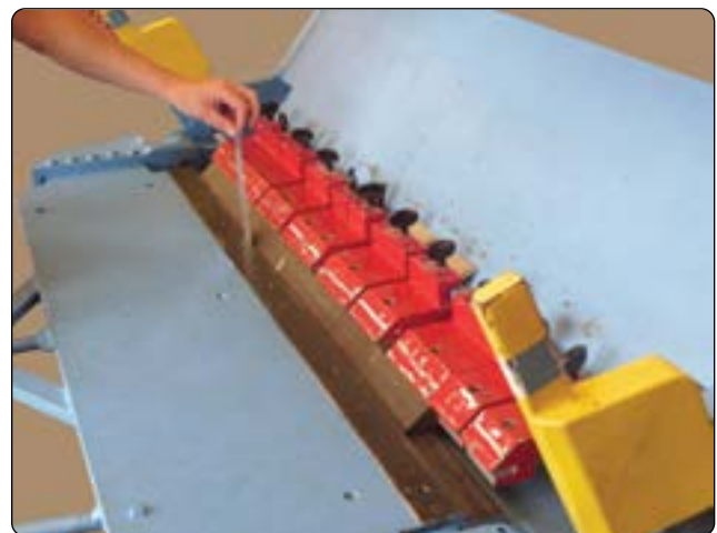
Figure 4-140. Brake nose gap adjustment with piece of material same thickness as part to be formed.
