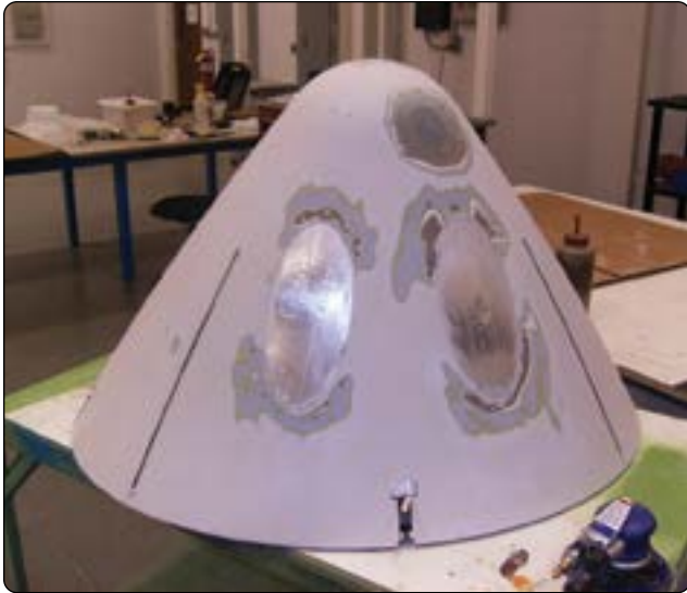
Figure 7-21. Damage to radome honeycomb sandwich structure.
