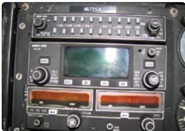
Figure 11-151. Panel-mounted LORAN units are now obsolete as LORAN signals are no longer generated from the tower network.
