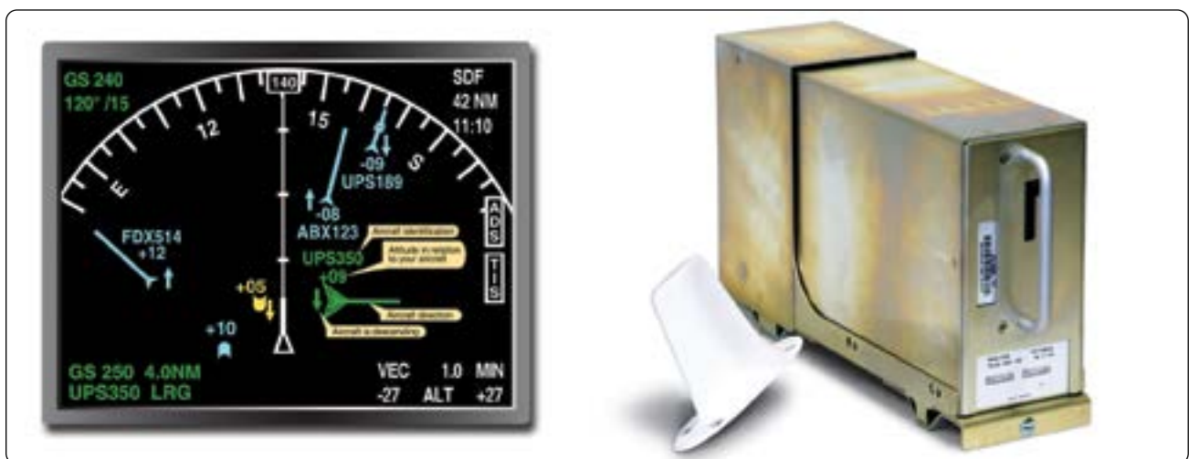
Figure 11-137. A flight deck display of ADS-B generated targets (left) and an ADS-B airborne receiver with antenna (right).
