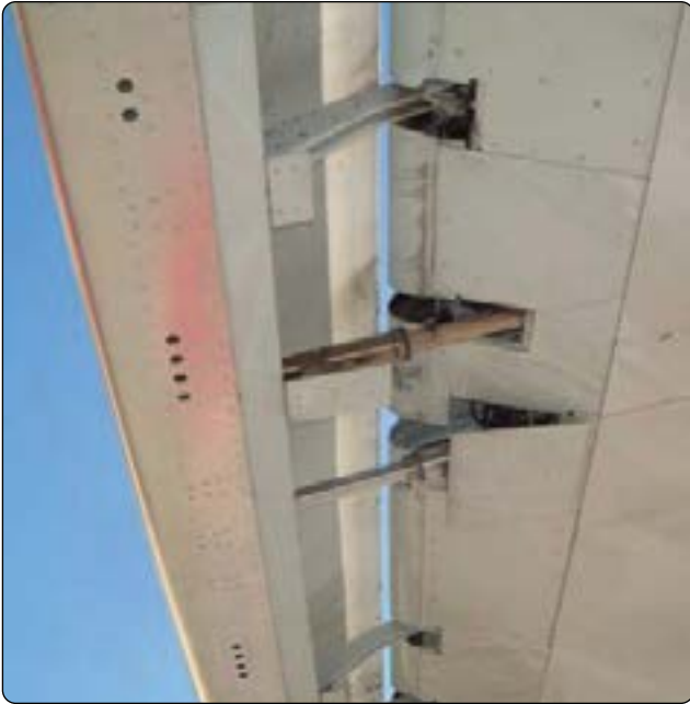
Figure 1-67. Air passing through the slot aft of the slat promotes boundary layer airflow on the upper surface at high angles of attack.
