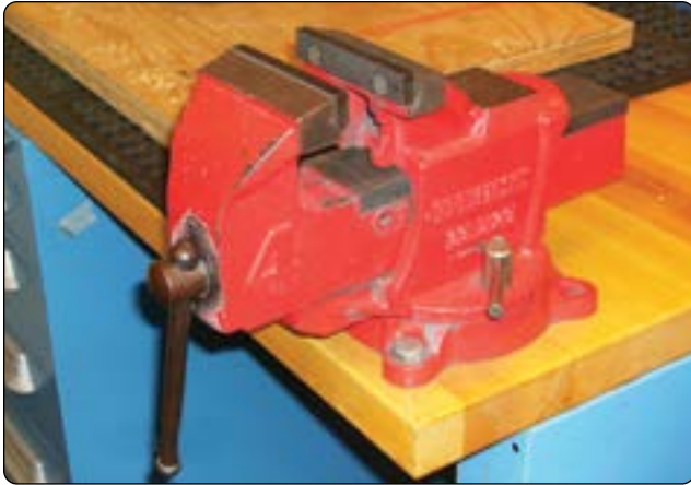
Figure 4-71. A utility vise with swivel base and anvil.
