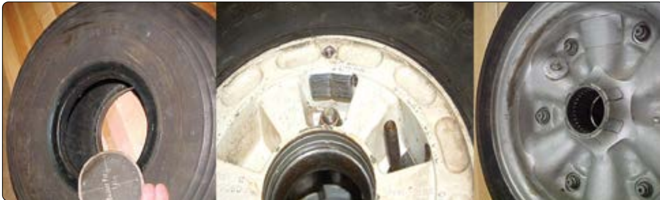
Figure 13-160. A tire balancing patch (left), adhesive wheel weights (center), and a bolted wheel weight (right) are all used to balance aircraft tire and wheel assemblies per the manufacturer's instructions.
