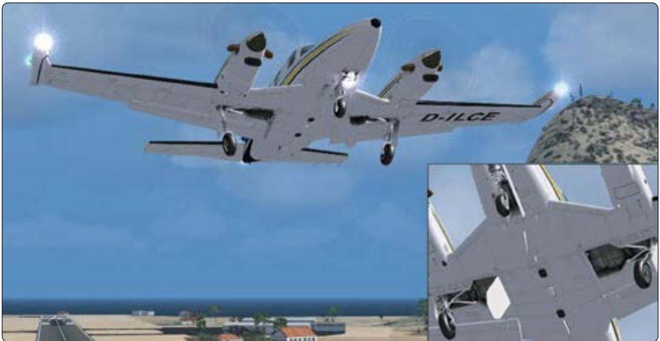
Figure 1-40. Engine nacelle incorporating the landing gear with the wheel well extending into the wing root.
