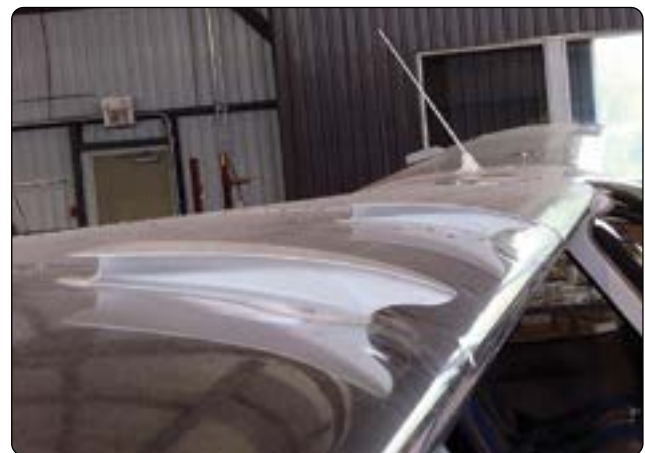
Figure 1-79. The Symphony SA-160 has two unique vortex generators on its wing to ensure aileron effectiveness through the stall.
