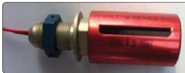
Figure 14-103. A float switch installed in a fuel tank can close the refueling valve when the tanks are full during pressure fueling of an aircraft. Other more sophisticated automatic shutoff systems exist.
