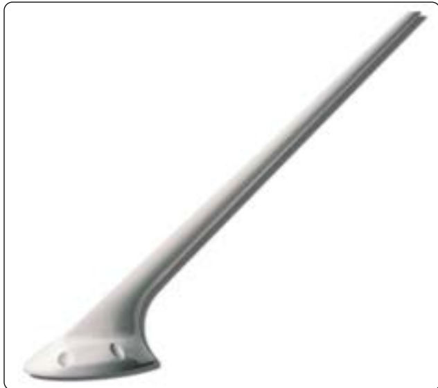
Figure 11-90. Many antenna are canted for better reception.
