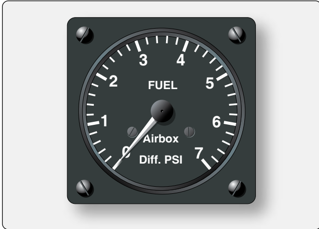
Figure 14-84. A differential fuel pressure gauge used on complex and high-performance reciprocating-engine aircraft compares the fuel inlet pressure to the air inlet pressure at the fuel metering device.
