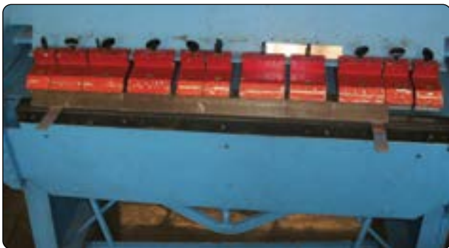
Figure 4-142. Brake alignment with two test strips 3 inches from each end.
