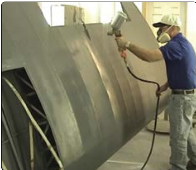
Figure 3-35. Applying a primer with UV blocking by spraying cross coats.
