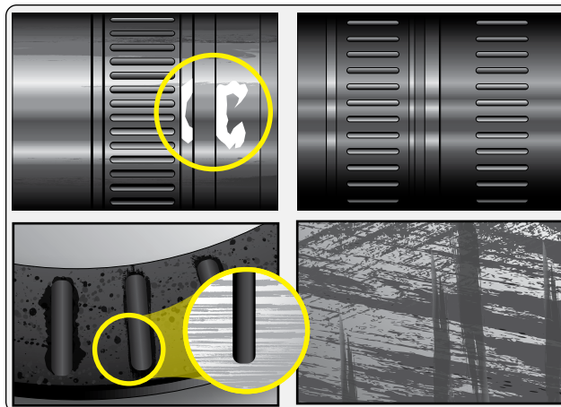
Figure 13-69. False brinelling is caused by vibration of the bearing while in a static state. Even with a static overload, it can force the lubricant from between the rollers and the raceway. Submicroscopic particles removed at the points of metal-to-metal contact oxidize. They work to remove more particles spreading the damage. This is also known as frictional corrosion. It can be identified by a rusty coloring of the lubricant.
