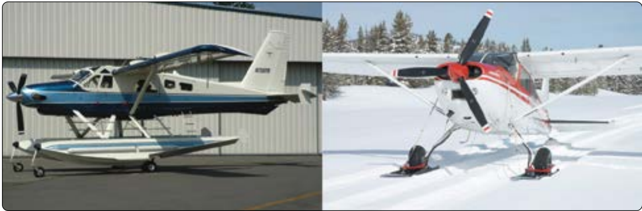
Figure 13-2. An amphibious aircraft with retractable wheels (left) and an aircraft with retractable skis (right).
