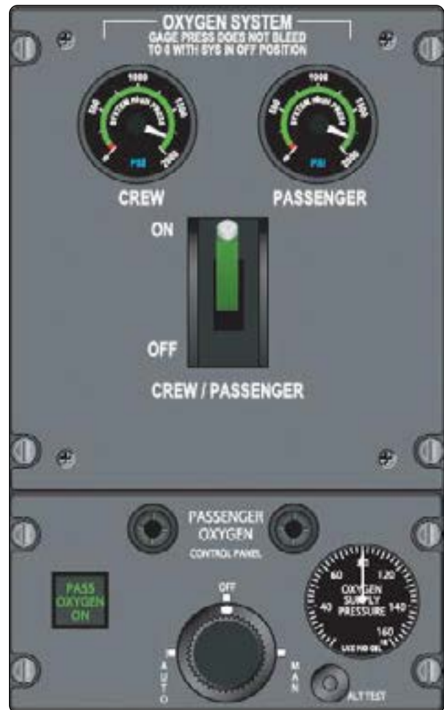
Figure 16-16. The crew can deploy passenger emergency continuous-flow oxygen masks and supply with a switch in the flight deck.
