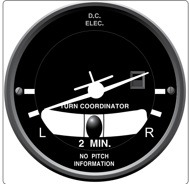
Figure 10-104. A turn coordinator senses and indicates the rate of both roll and yaw.
