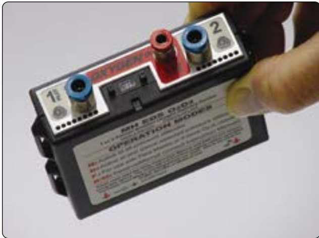
Figure 16-24. A portable two-person electronic pulse-demand (EPD) oxygen regulating unit.
