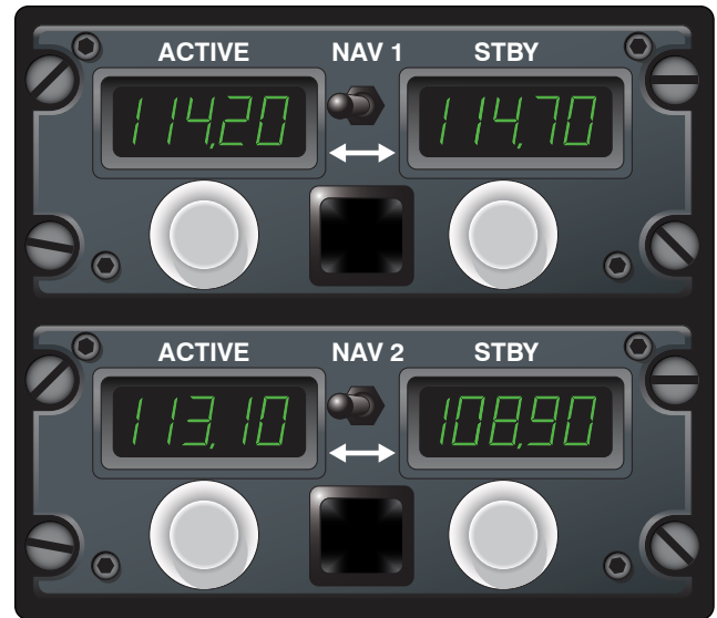
Figure 11-100. An airliner VOR control head with two independent NAV receivers each with an active and standby tuning circuit controlled by a toggle switch.
