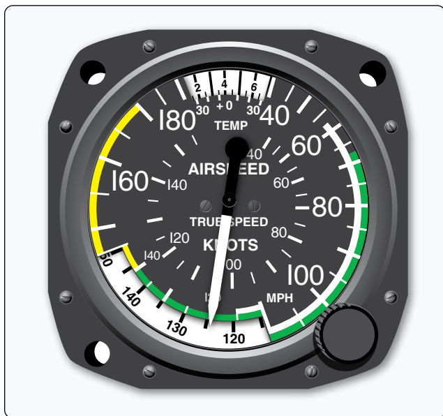
Figure 10-43. An analog true airspeed indicator. The pilot manually aligns the outside air temperature with the pressure altitude scale, resulting in an indication of true airspeed.
