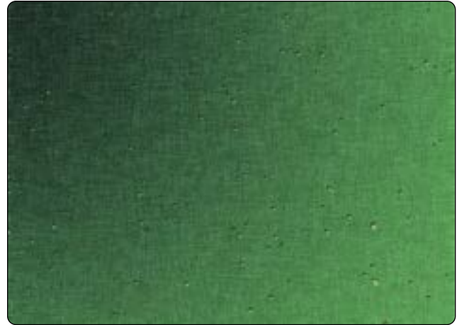
Figure 8-15. Example of pinholes.
