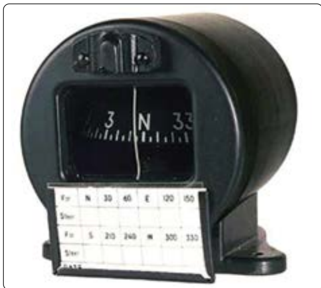
Figure 10-139. A magnetic compass with a deviation correction card attached, on which the results of swinging the compass should be recorded.
