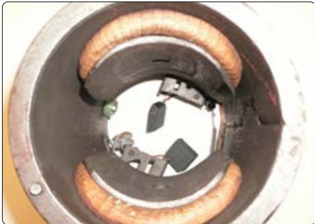
Figure 9-46. Generator field frame.
