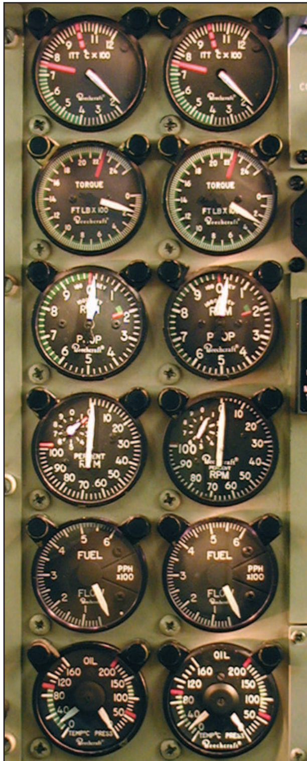
Figure 14-7. Engine instruments—split shaft/free turbine engine.
