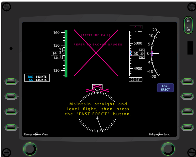
Figure 2-8. A PFD indicating a failed AHRS.
