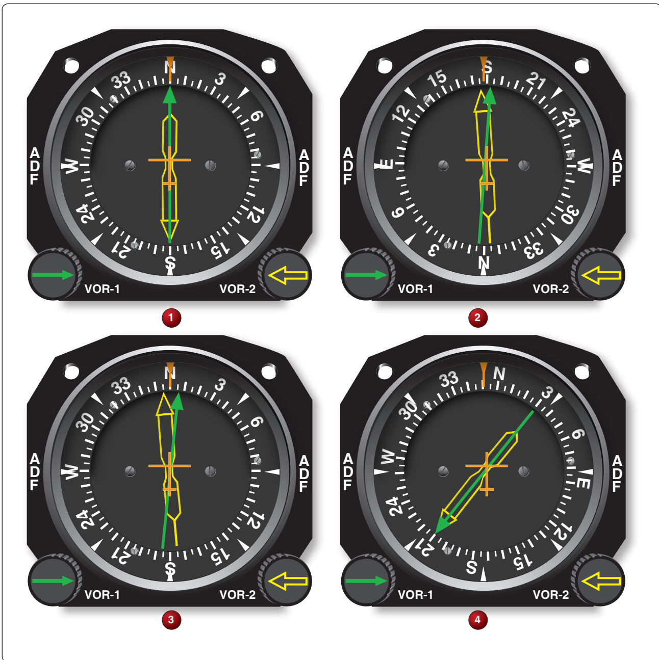
FIGURE 82.—Dual VOR System, Accuracy Check.
