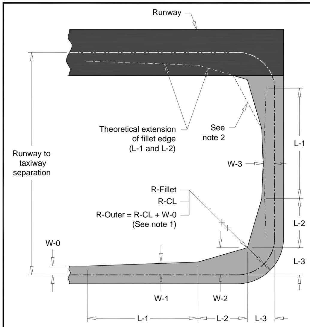
**Note 1:** Radii of the fillet and the taxiway centerline are not concentric. The radii of the centerline and the outer pavement edge are concentric.
