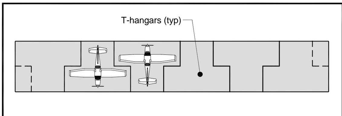
**Note:** The standard T-hangar configuration offers the advantage of minimizing the structure depth when length is not a controlling factor.
