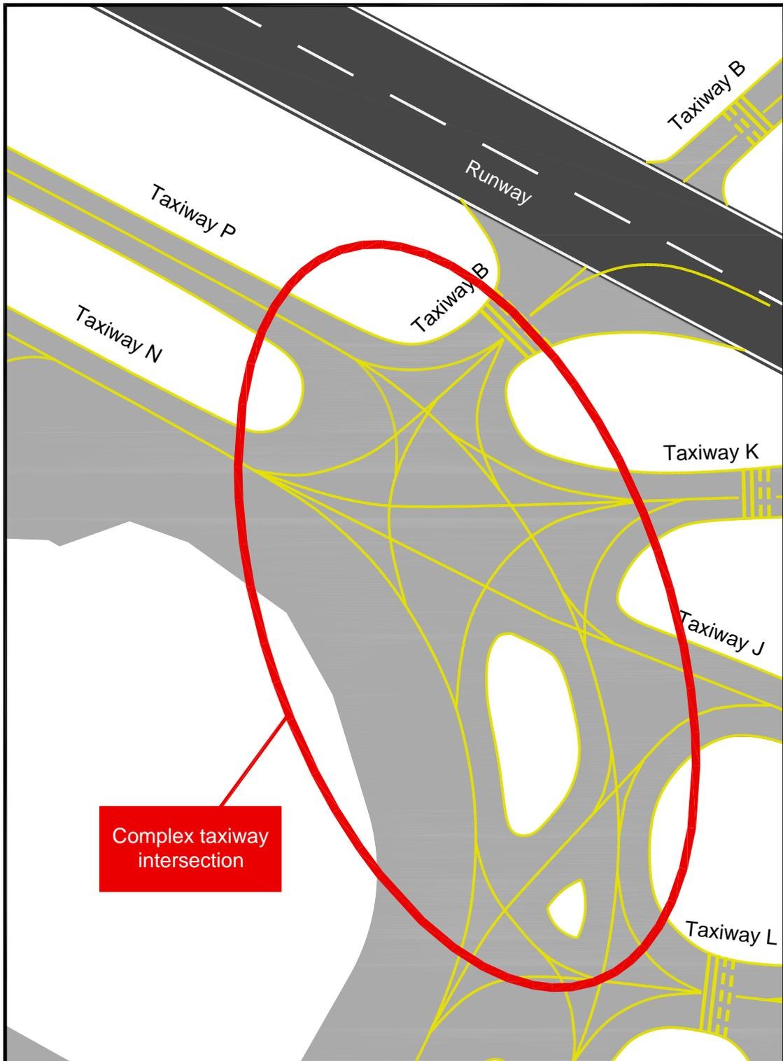
**Figure J-17. Aerial Image of Complex Taxiway Intersection Exceeding the “Three-Path” Concept**
