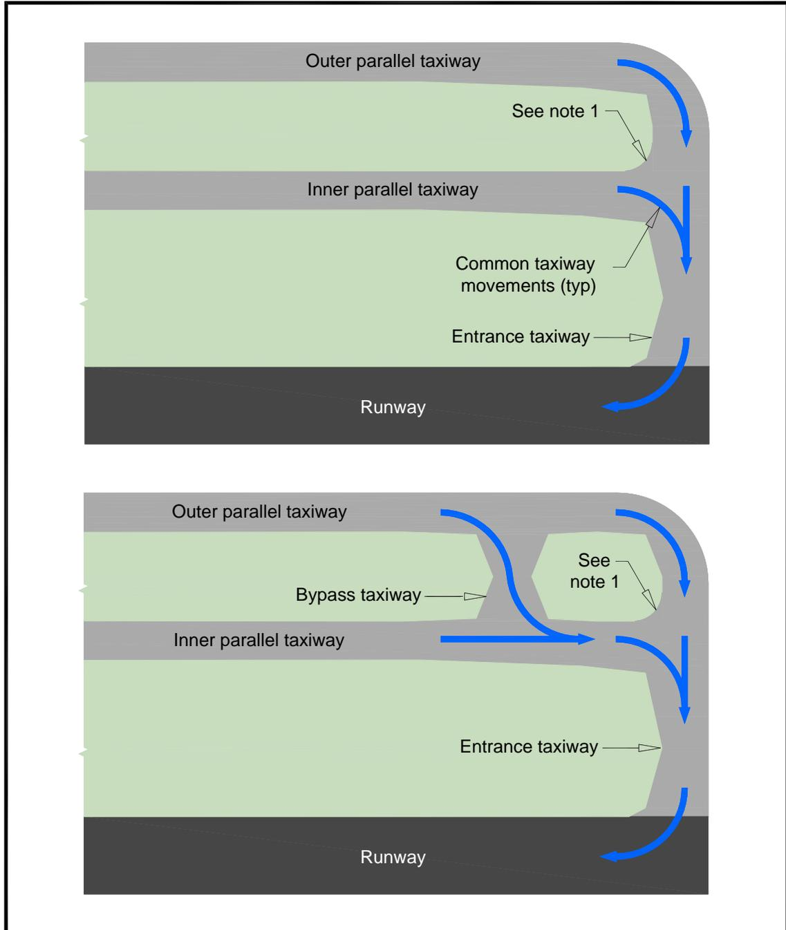
**Note 1:** Providing a centerline radius marking and standard fillet for the uncommon turn from the connecting taxiway to the inner parallel can create a risk for a taxiway departure. Refer to paragraph 4.6 for additional guidance on reducing this risk.
