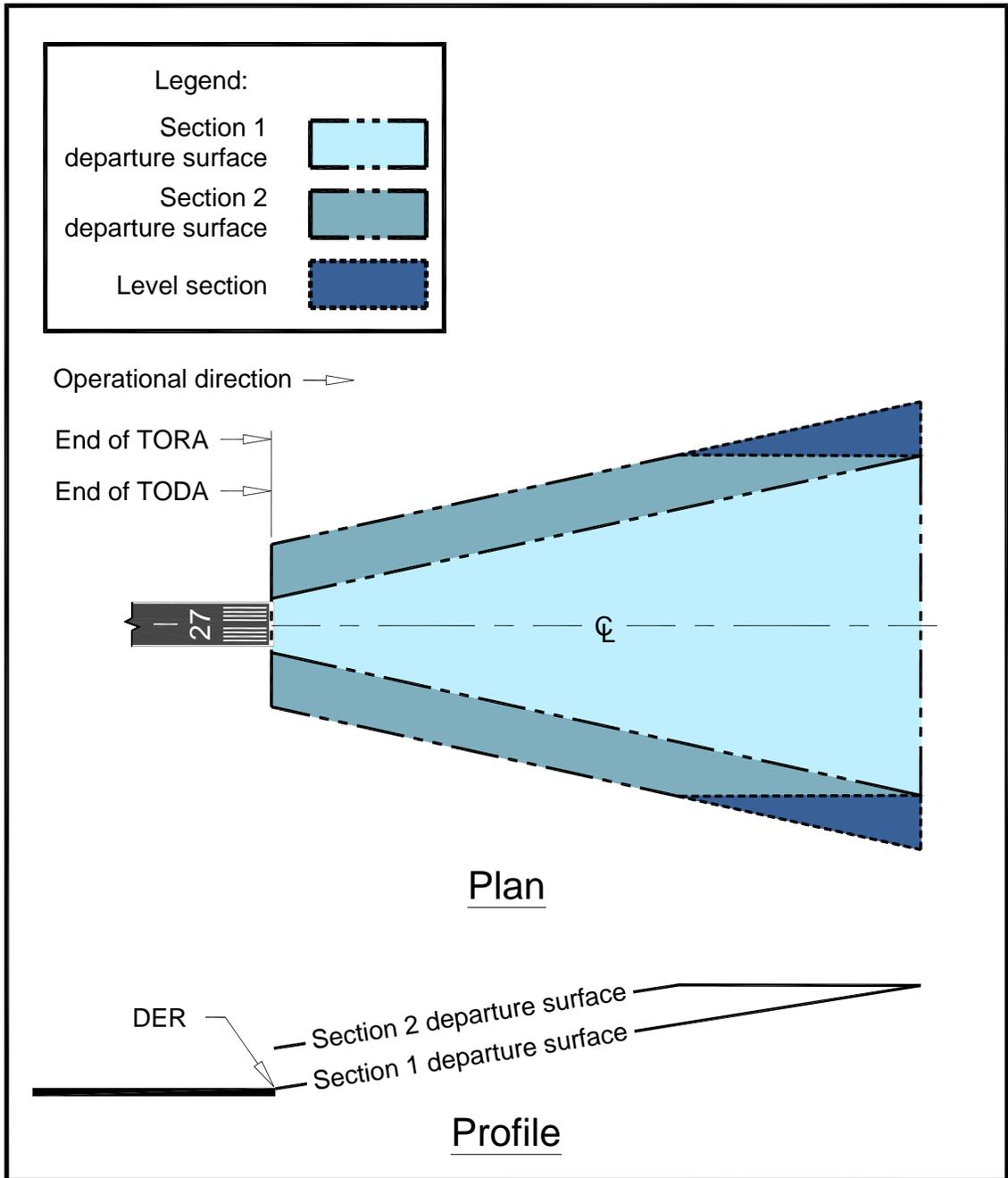
**Figure H-7. Extended TODA with Clearway – Typical TORA**
