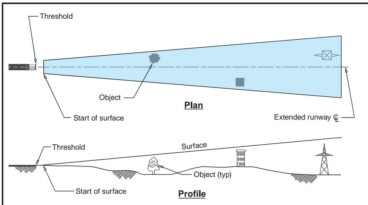
**Note 1:** The starting elevation of the approach slope is the elevation of the runway threshold.
