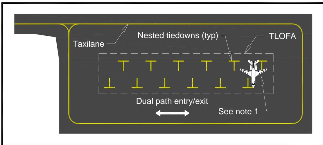
**Note 1:** Nested parking position can provide flexibility by accommodating parking of larger aircraft. Ensure tiedowns for smaller aircraft do not pose a hazard to larger aircraft.
