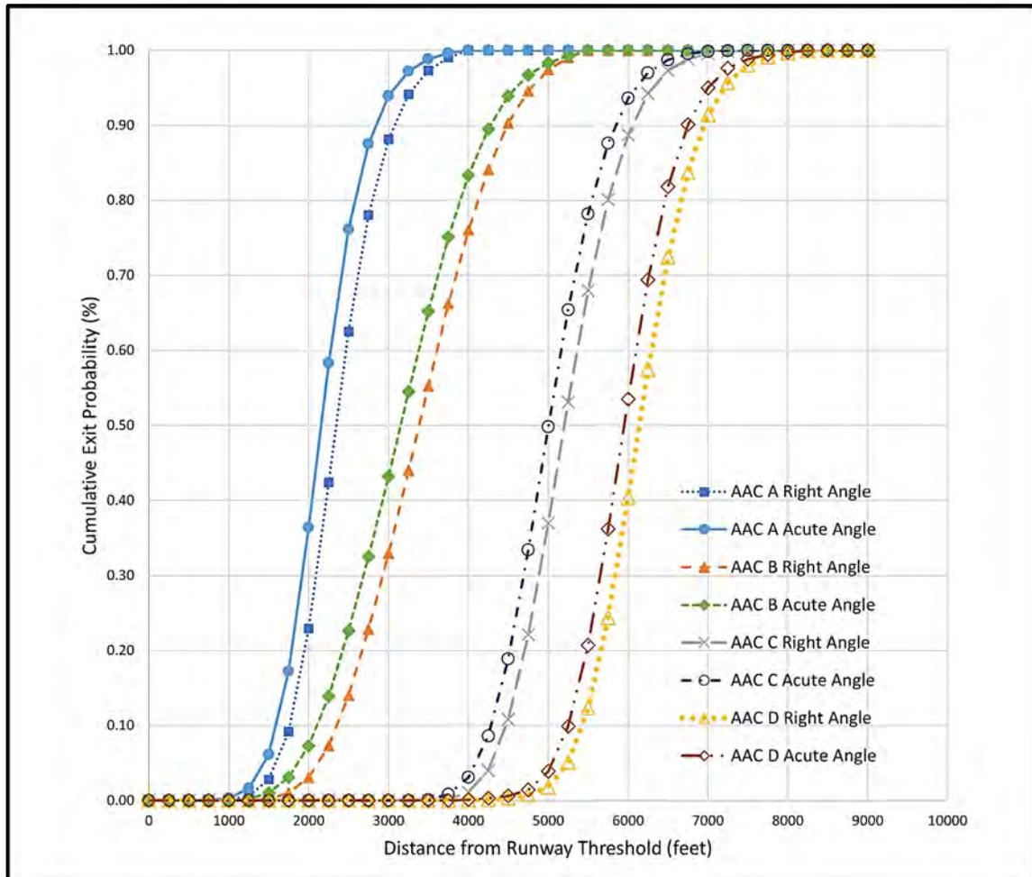
**Note:** Figure 4-17 provides a simplified method using cumulative exit probability distribution for airports with an elevation under 2,000 feet (610 m) MSL. This method is appropriate to use for the initial, conceptual planning. Analysis using REDIM-V3 to incorporate airport specific variables (e.g., elevation and fleet mix) is preferred, particularly when considering proper placement of high-speed exits.
