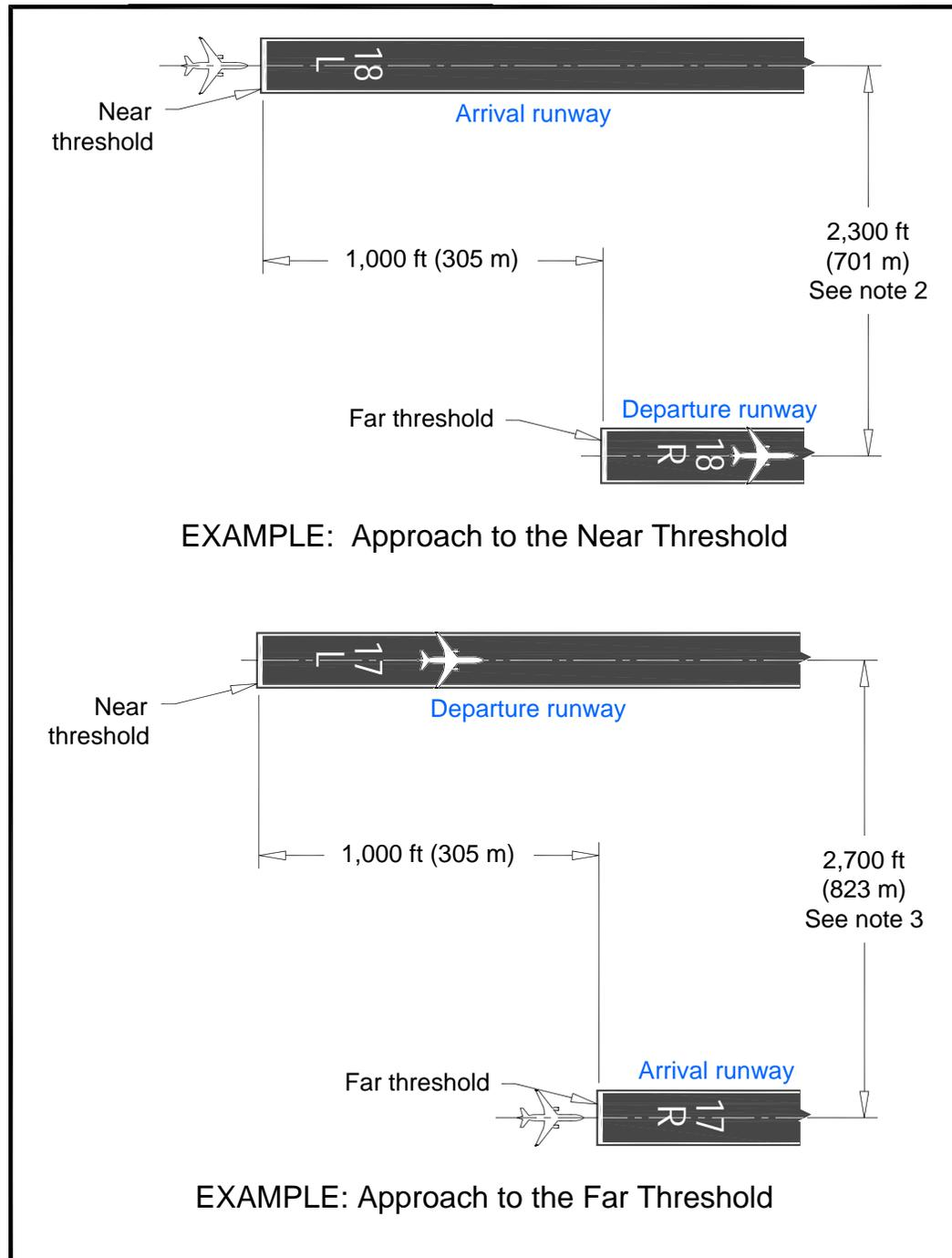
**Note 1:** Figure 3-18 illustrates parallel runway separation adjustments from the standard 2,500 ft (762 m) used with even thresholds for simultaneous radar-controlled mixed operations (arrival to one runway and departure on the other runway).
