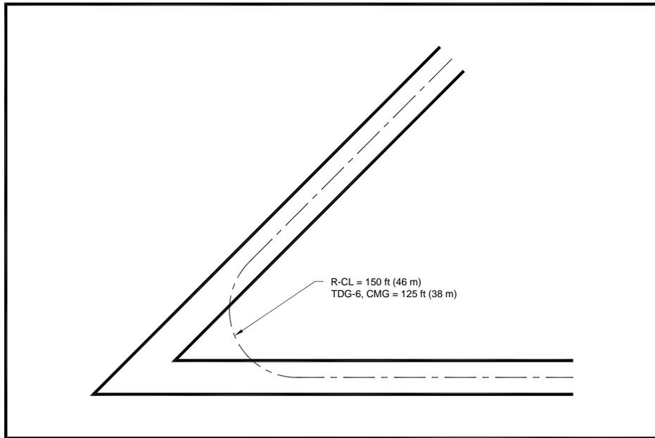
J.2.11.3 As shown in [Figure J-4](#), model the track of the main gear of the longest CMG and widest MGW using an offset equal to the TESM. For TDG 6, the TESM is 14 feet (4.3 m).
