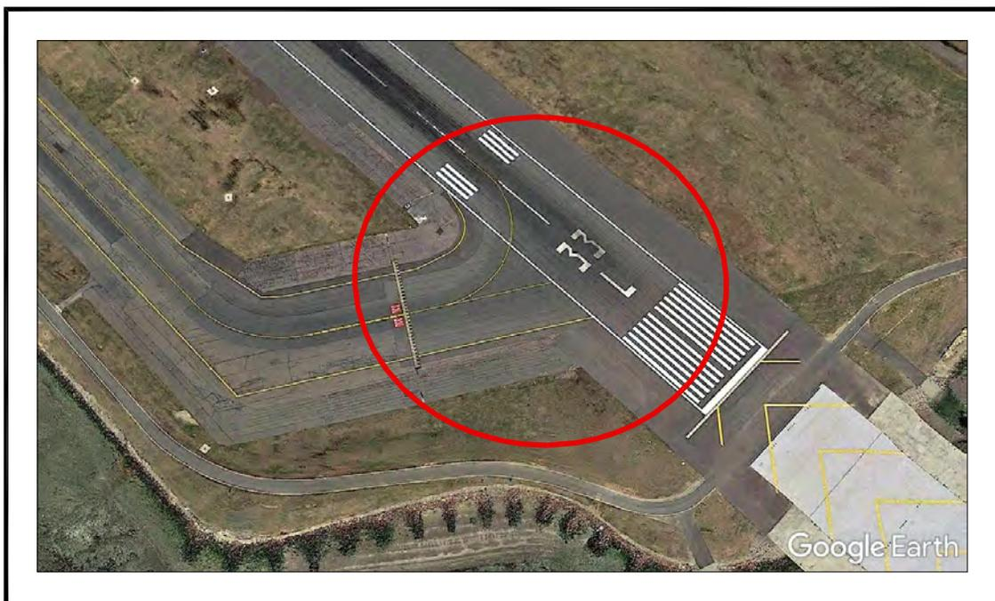
**Note:** A pilot at the holding position has an enhanced viewing range of the approach area but a limited field of view down the runway.
