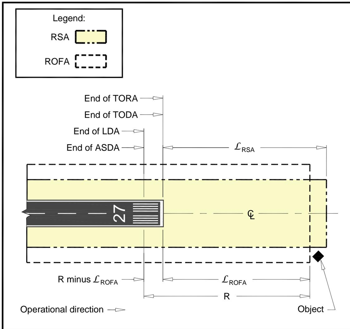
**Note 1:** When a stopway exists, see [Figure H-11](#) for the departure end of the ASDA.
