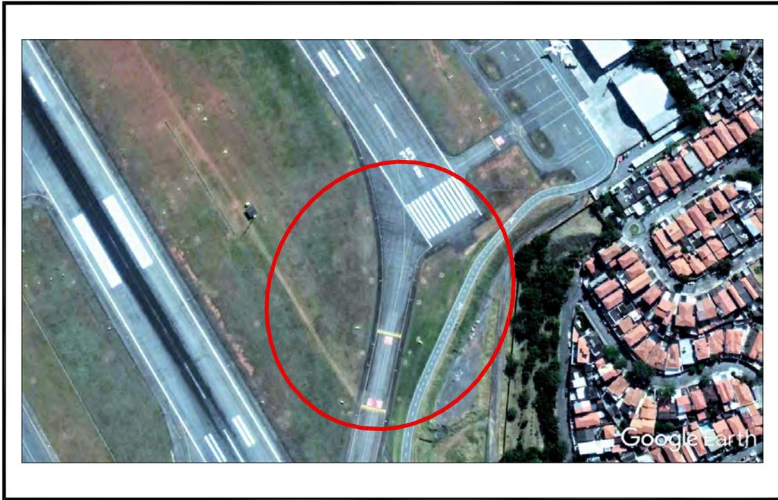
**Note:** A pilot at the holding position has an enhanced viewing range of the runway but a limited field of view in the approach area.
