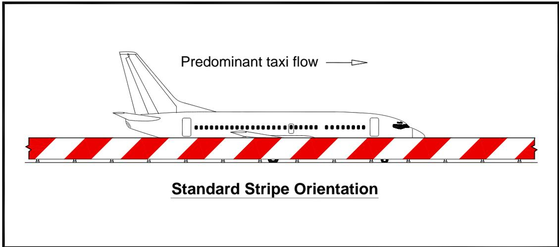
**Note:** The front panel of the screen is retroreflective red and white (see paragraph [D.2.4.3](#)).
