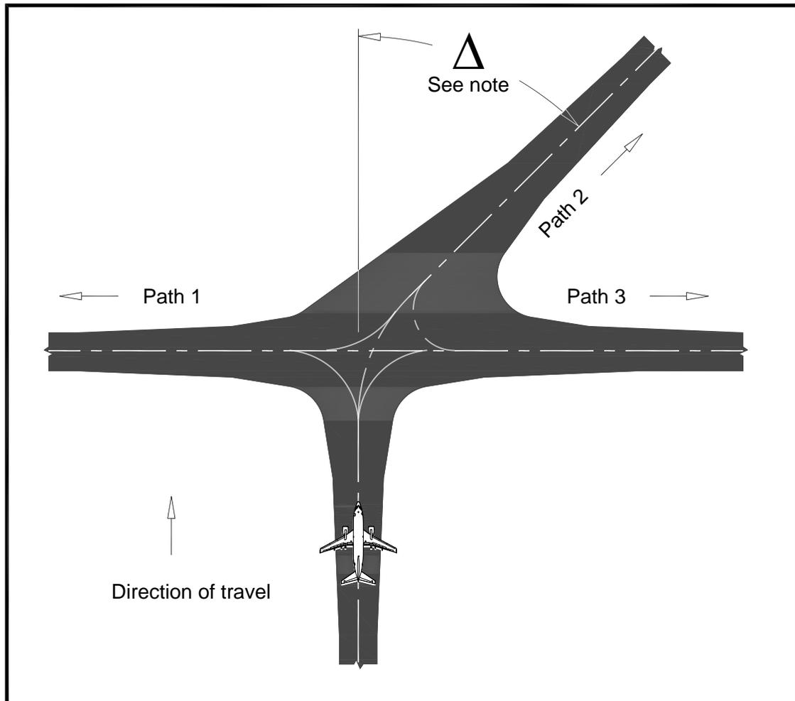
**Note:** The angle ( $\Delta$ ) is measured from the initial direction of travel.
