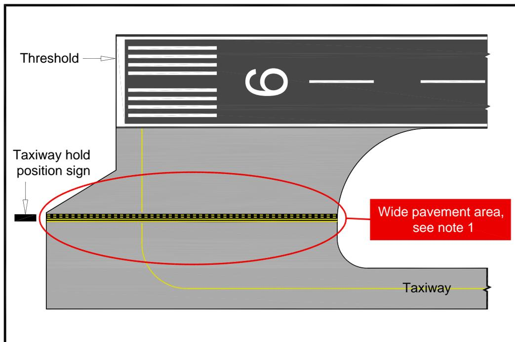
**Note 1:** The wide distance of the holding bay places the vertical signs outside of the pilot's normal viewing range.
