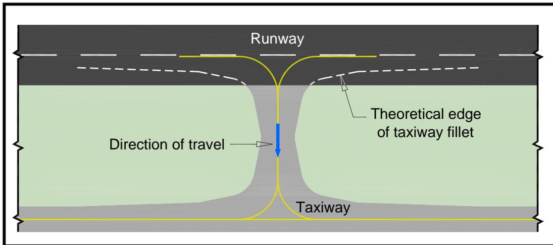
**Figure 4-21. High-Speed Exit Separation**
