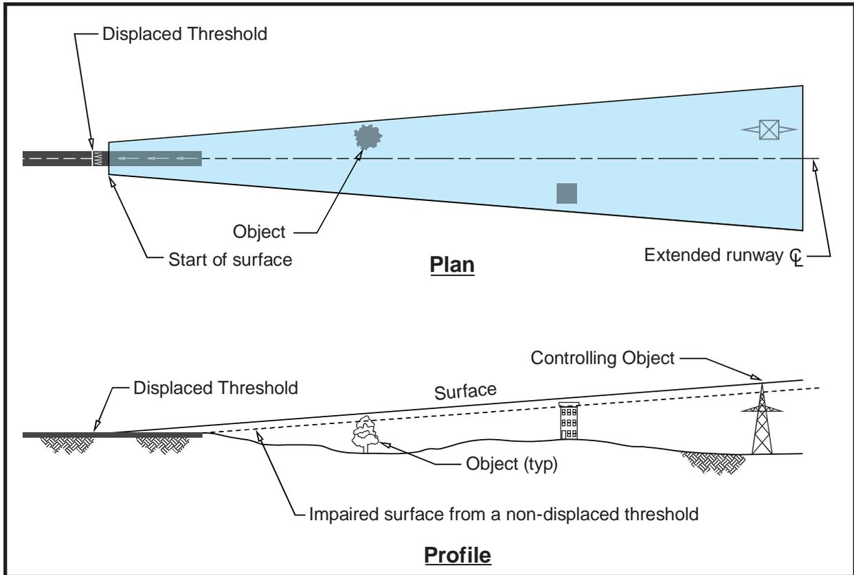
**Note 1:** The starting elevation of the approach slope is the elevation of the runway displaced threshold.
