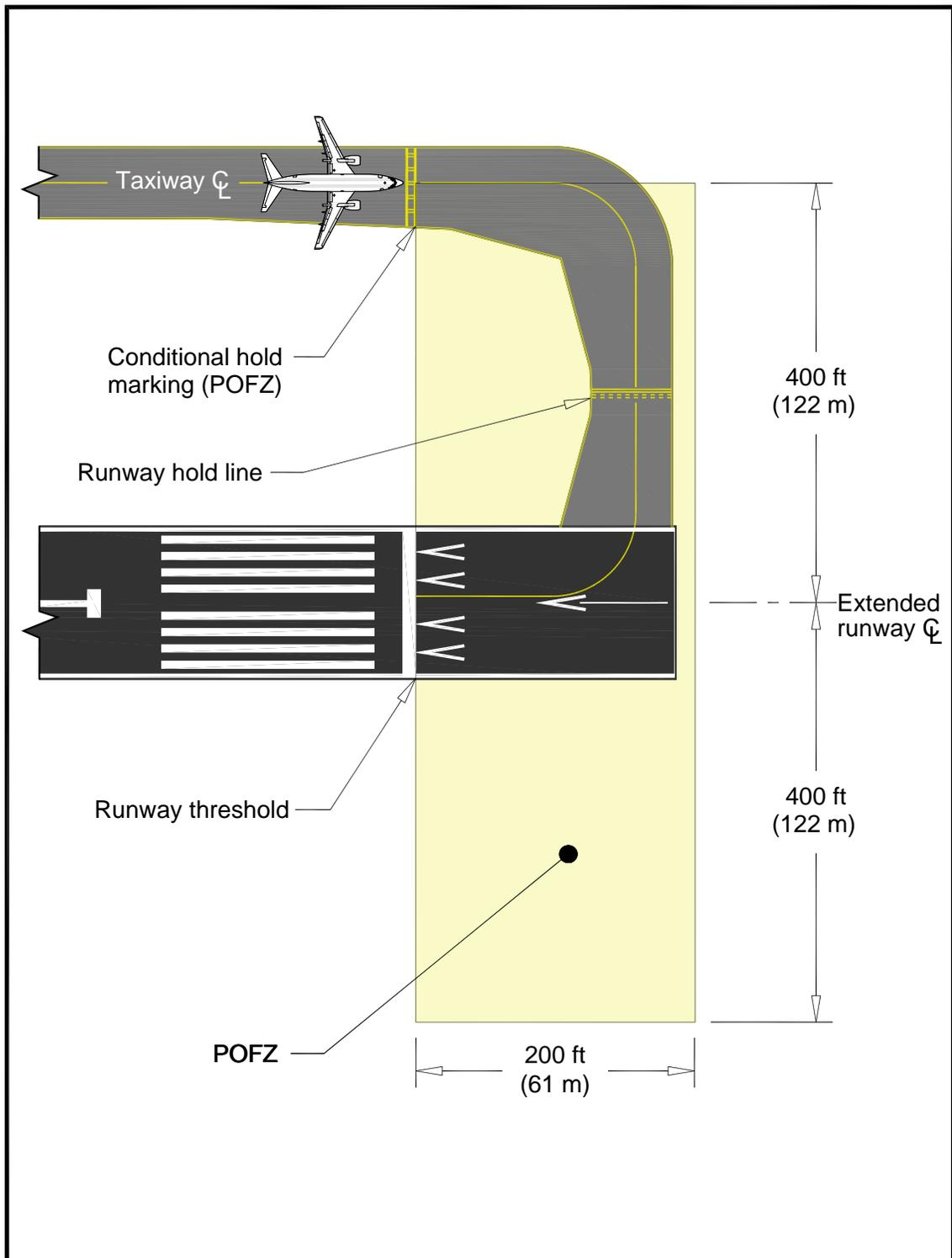
**Note 1:** Two hold lines are necessary, as the POFZ is only in effect during instrument meteorological conditions.
