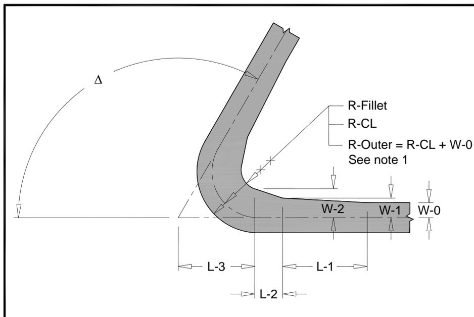
**Note 1:** Radii of the fillet and the taxiway centerline are not concentric. The radii of the centerline and the outer pavement edge are concentric.
