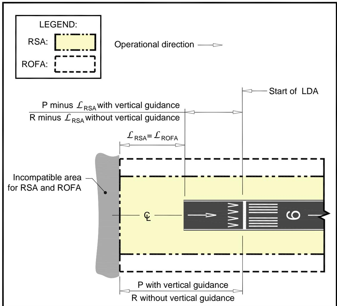
**Note 1:**  $\mathcal{L}_{\text{RSA}}$  and  $\mathcal{L}_{\text{ROFA}}$  denote the effective lengths of the RSA and ROFA beyond the runway end, respectively.
