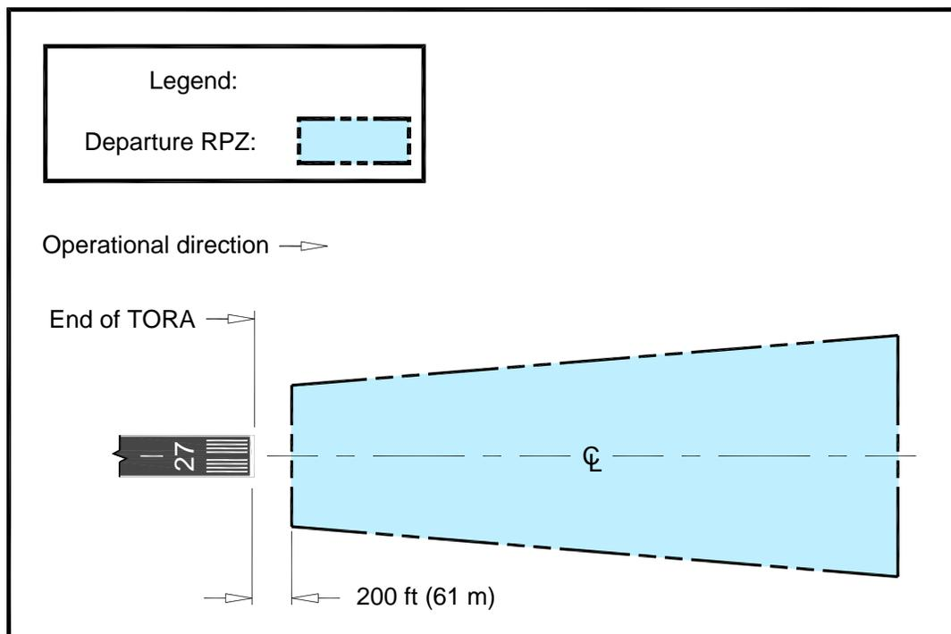
**Figure H-3. Modified Departure End of TORA due to Incompatible Land Use Within RPZ**
