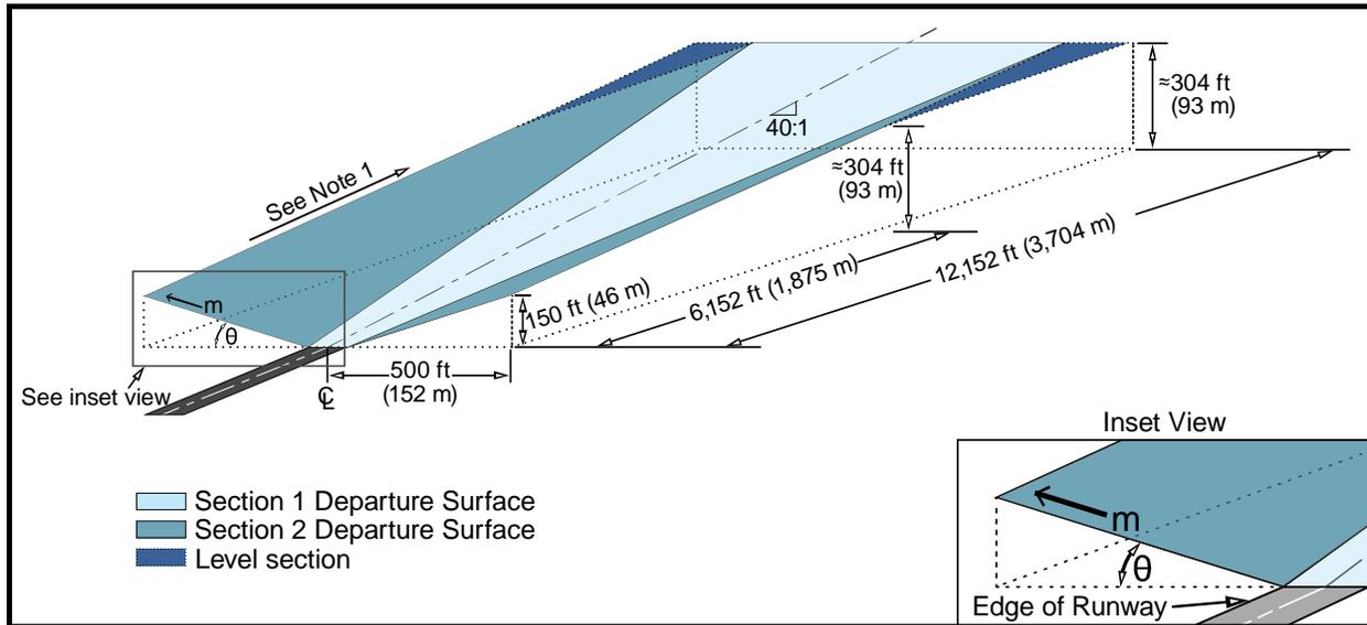
**Note 1:** The outer edge of the Section 2 Departure Surface has a slope of 40:1.
