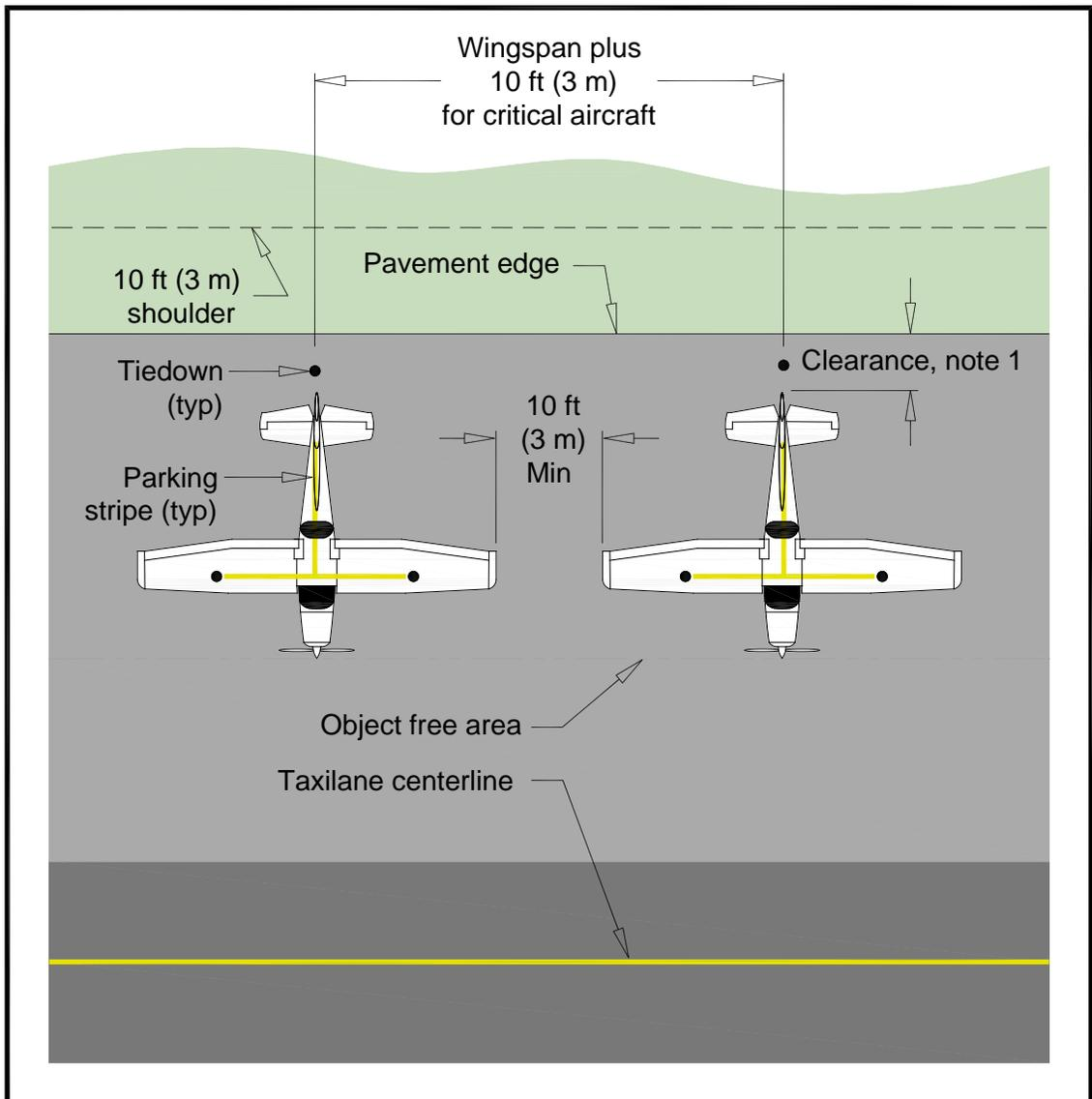
**Note 1:** Provide sufficient space between the pavement edge and the tail to permit pilots to walk around aircraft during preflight check.
