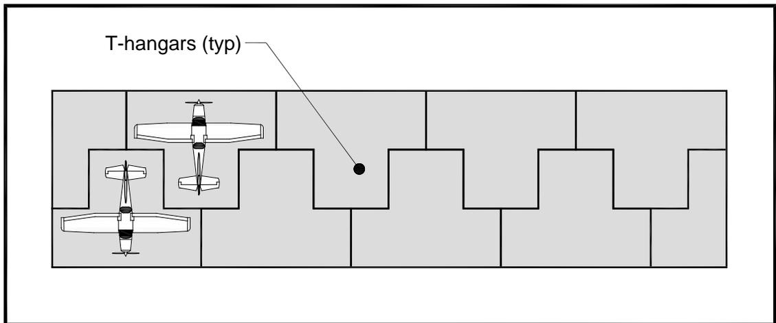
**Note:** The nested T-hangar configuration offers the advantage of minimizing the structure length when depth is not the controlling factor.
