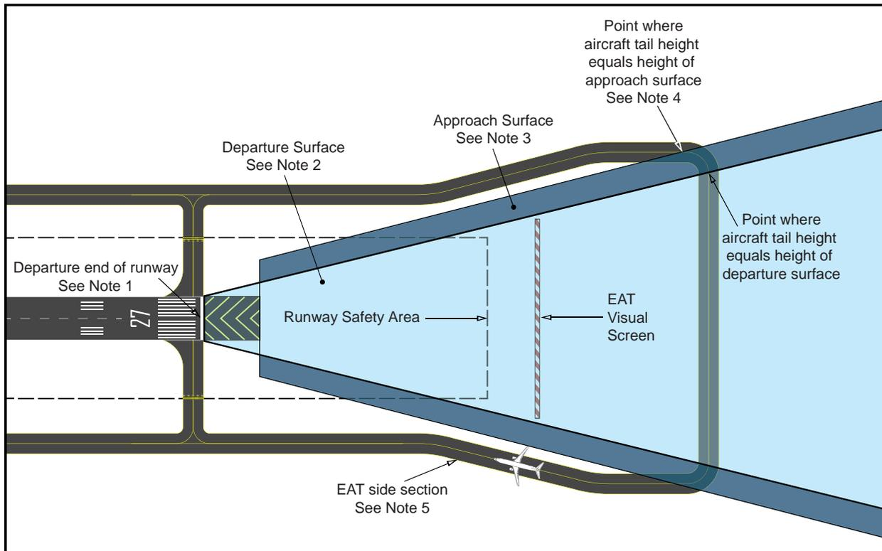
**Note 1:** Assumes all centerline elevations are equal to the elevation of the departure end of the runway.
