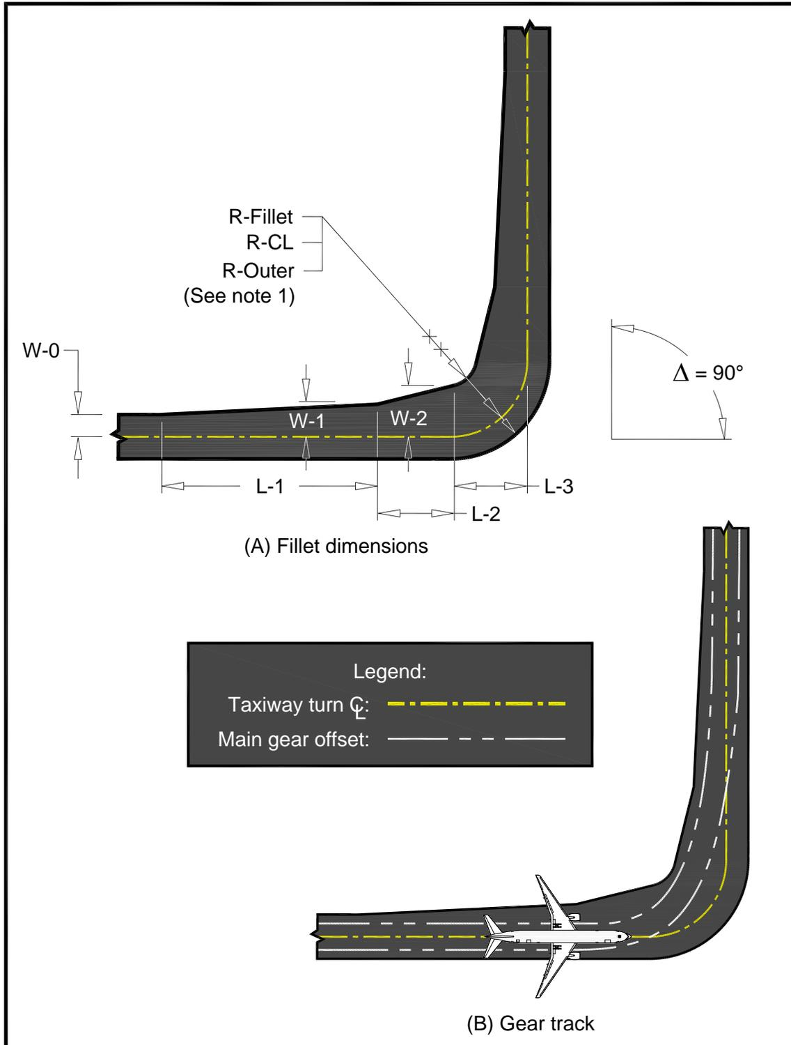
**Note 1:** Radii of the fillet and the taxiway centerline are not concentric. The radii of the centerline and the outer pavement edge are concentric.
