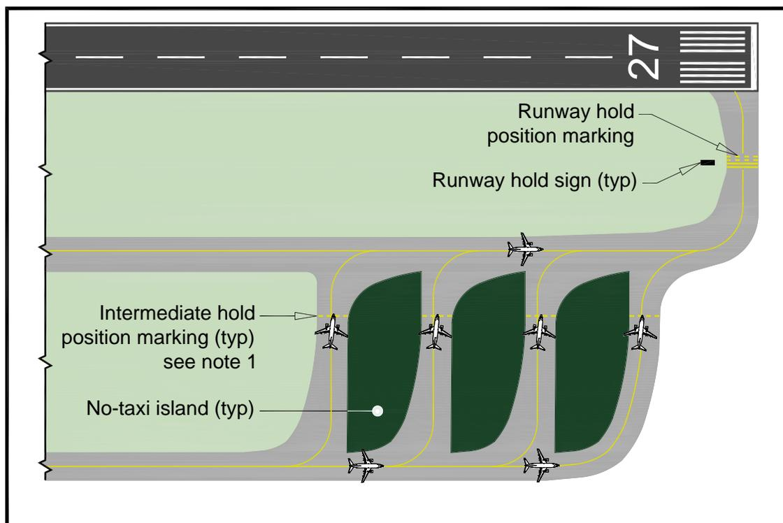
**Note 1:** Locate intermediate hold lines at the outer limit of the inner TOFA.
