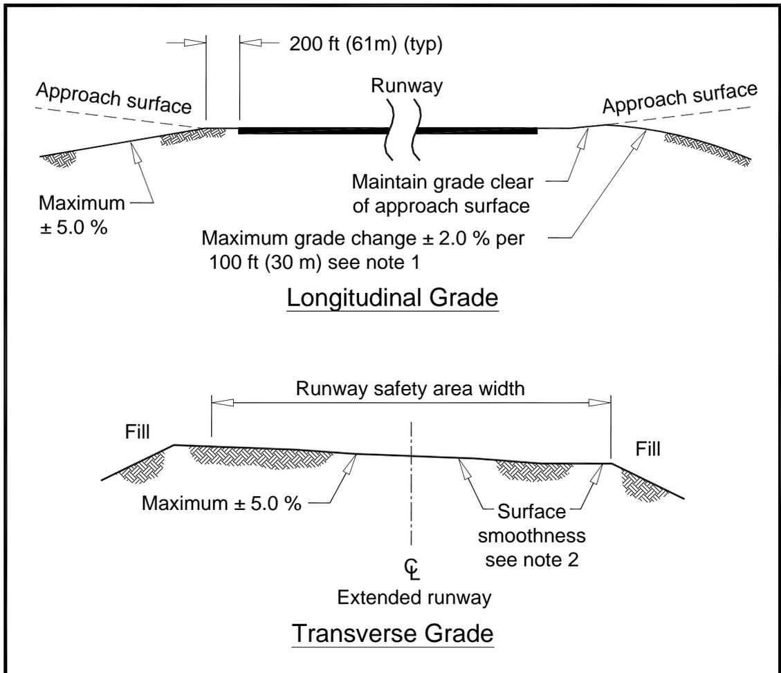
**Note 1:** Use a vertical curve to transition between longitudinal grade changes.
