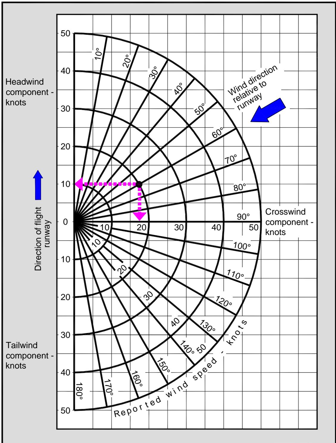
**Note:** Example: Wind speed 20 knots angle between runway and direction of wind – 60° crosswind component – 17 knots. Headwind component – 10 knots.
